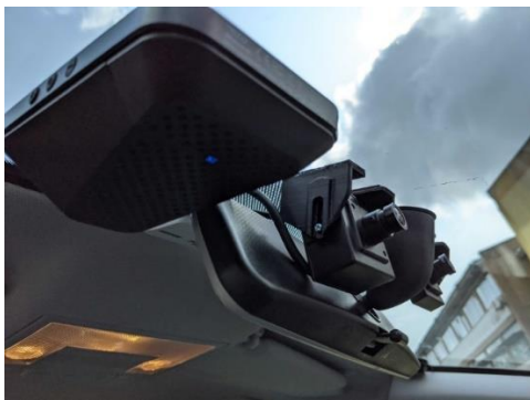
Figure 19: Mobileye and CardioDashcam fitted in a vehicle's windshield.
