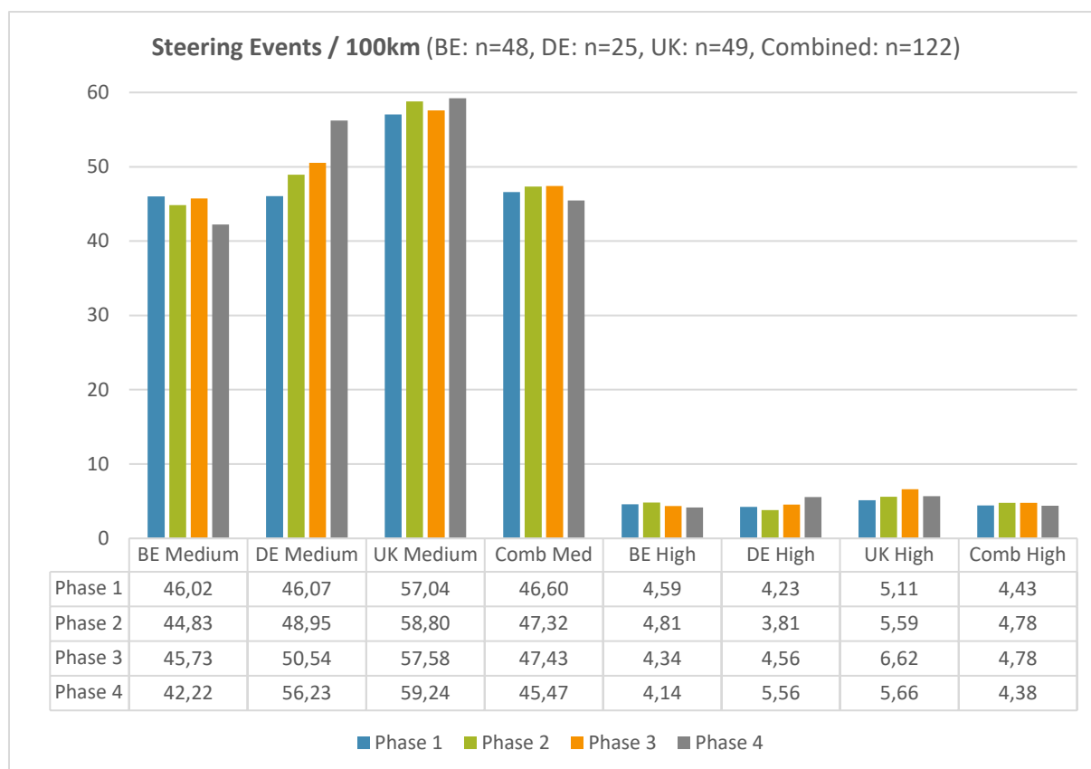
Figure 35: Medium and High steering events / 100km per country and per phase (cars)
