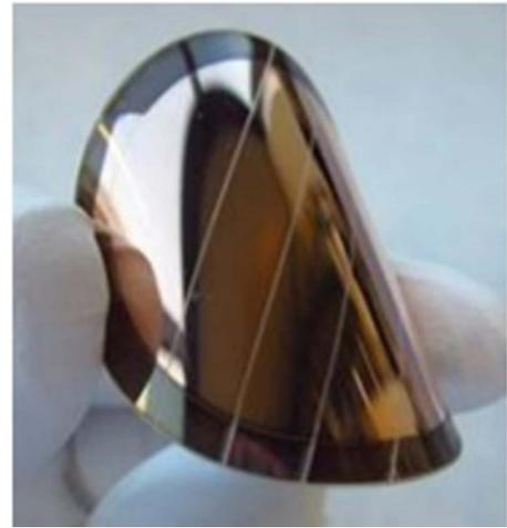
**Figure 13.** Flexible perovskite photovoltaic.
