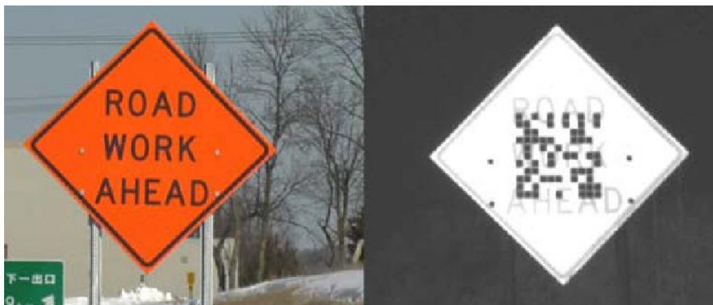
Figure 8 Example of visible and Near-IR view of QR code (Source: [58])
