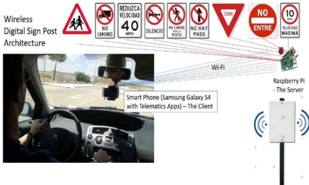
Figure 14 Programmable wireless digital traffic signpost architecture (Source: [71])
