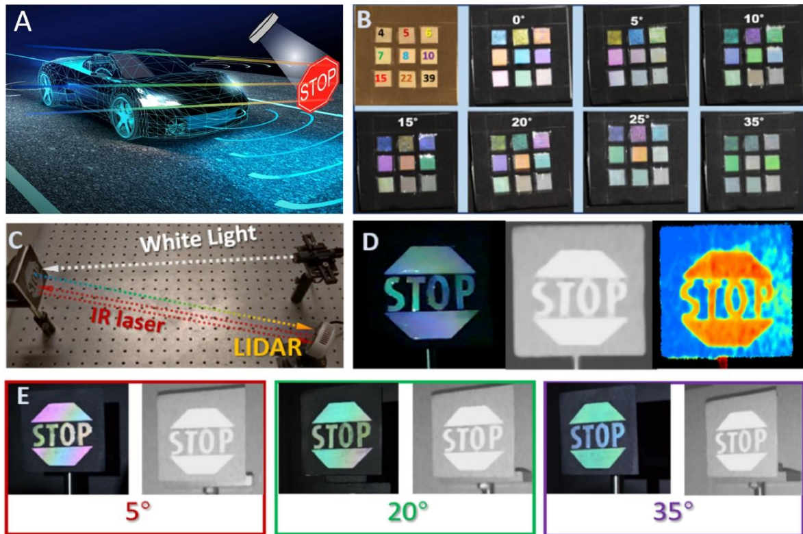
Figure 13 Visible and IR reflective road sign based on the microscale concave interfaces structures technology, under different light illumination conditions (Source: [69])
