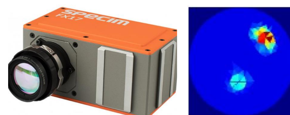
Figure 7: Near-infrared spectroscopy (NIR) of remaining coating inclusions in handsheets from recycled pulp
