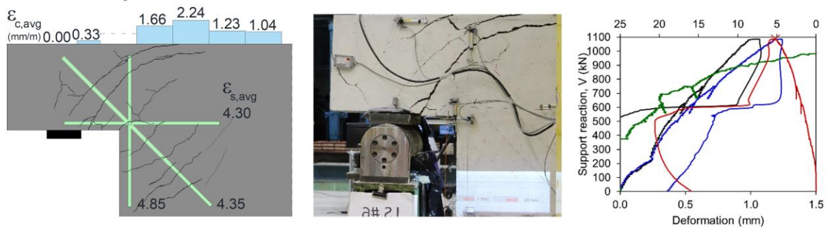
(h) Beam 4-DL8: left – crack pattern near peak load (1088 kN), middle – after failure, right – support reaction vs. crack components at the re-entrant corner
