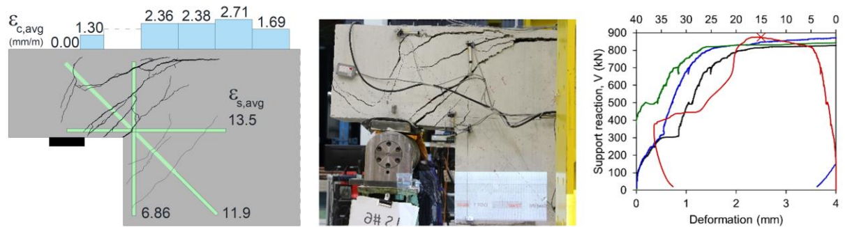
(f) Beam 3-DL6: left – crack pattern near peak load (875 kN), middle – after failure, right – support reaction vs. crack components at the re-entrant corner
