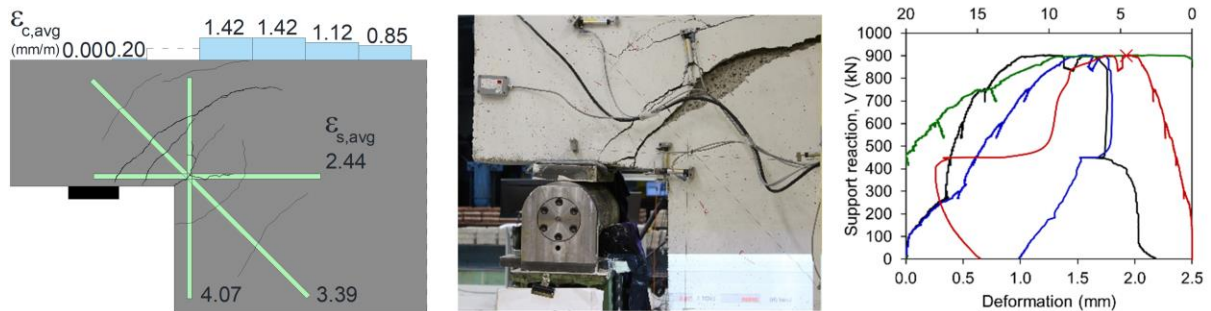
(g) Beam 4-DL7: left – crack pattern near peak load (900 kN), middle – after failure, right – support reaction vs. crack components at the re-entrant corner
