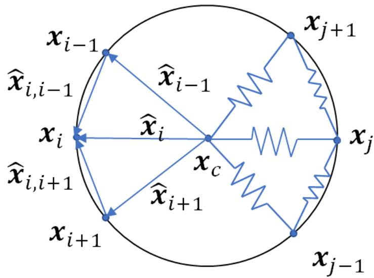
Fig. 2: A schematic of the distribution of the nodal points. The equilibrium shape is maintained by a collection of springs, from [1]
