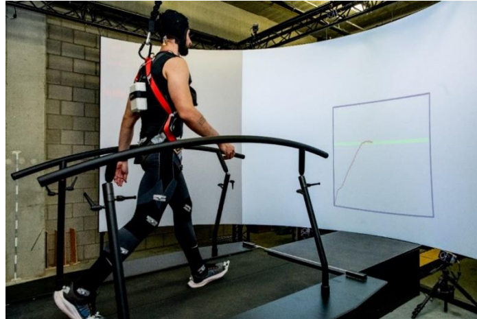
Figure 2. Gait Real-Time Analysis Interactive Lab with real-time visual feedback on walking speed.
