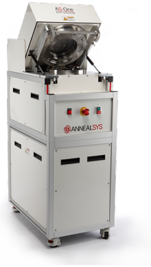
Figure 1.2: Annealsys AS-One furnace used for selenization of CIGS samples[4]
