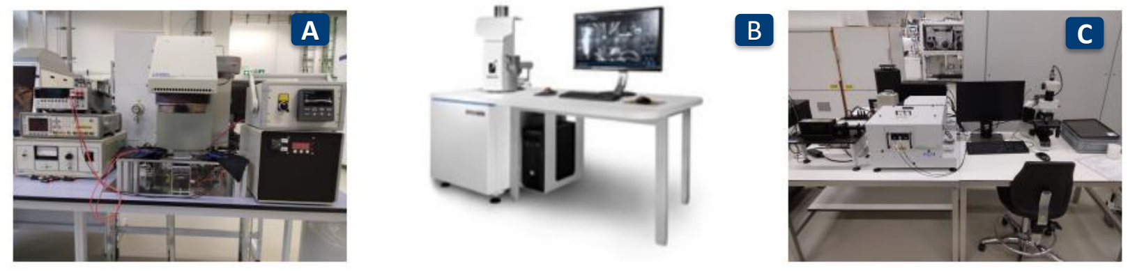
Figure 5: Characterization devices with A) photo-luminescence microscope (PL), B) Scanning electron microscope (SEM), C) oriel IV-setup
