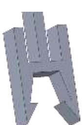
Fig. 2: Hoogfrequente resonator (48 mm x 26mm)
