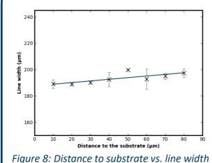
Figure 8 shows a **positive linear relationship** between substrate distance and line width when printing with a **200 µm nozzle**. As distance increases from **10**  $\mu$ m to **80**  $\mu$ m, line width grows from 188.8 ± 1.0 µm to 197,5 ± 3,2 µm. This emphasises the importance of accurate distance control to print consistent and precise lines
