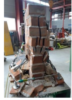
Figure 16 : Failure wall after compression, side
