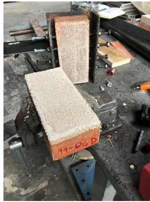
Figure 23 : Failure of the bed joint 1
