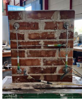
Figure 14 : Instrumented wall, back side
