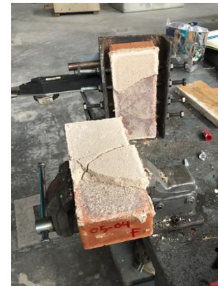
Figure 24 : Failure of the bed joint 2
