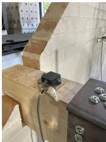
Figure 65 : Accelerometer placed on the purlin
