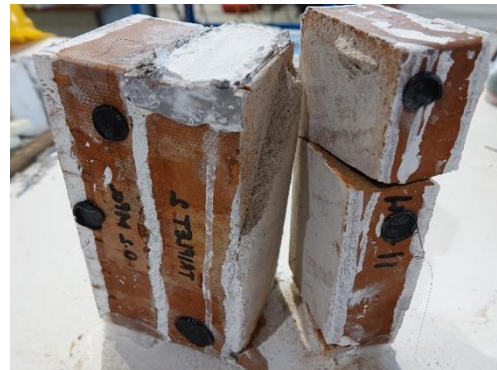
Figure 35 : fully formed crack after testing the shear strength
