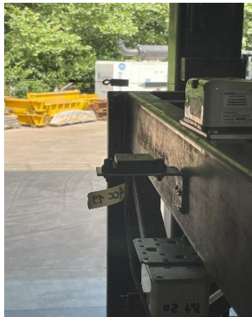
Figure 68 : Accelerometer applied on the instrumentation frame
