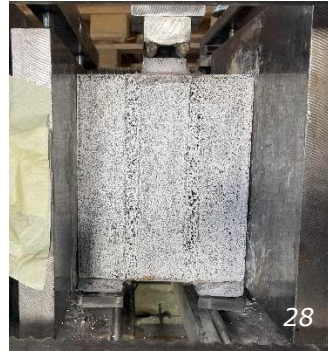
Figure 27 : Applied loads during shear tests conducted on triplets
