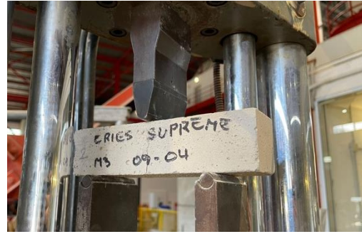
Figure 5 : Failure crack of the mortar
