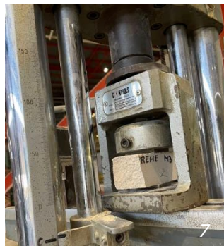
Figure 6 : compressive strength specimens after testing flexural strength
