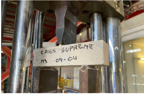
Figure 4 : Test setup determination of flexural strength
