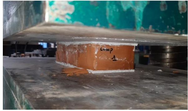
Figure 10 : Failure of the unit
