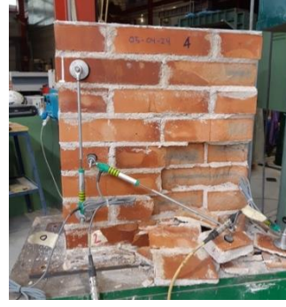
Figure 15 : Failure wall after compression, front side
