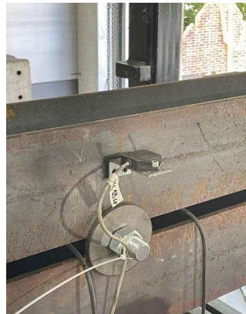
Figure 69 : Accelerometer located on the upper steel beam of the setup frame
