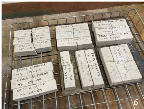
Figure 6 : compressive strength specimens after testing flexural strength
