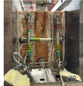
Figure 28 : DIC instrumentation adopted to determine the shear strength, front side
