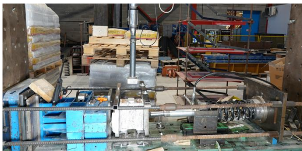
Figure 27 : test set-up used for shear strength
