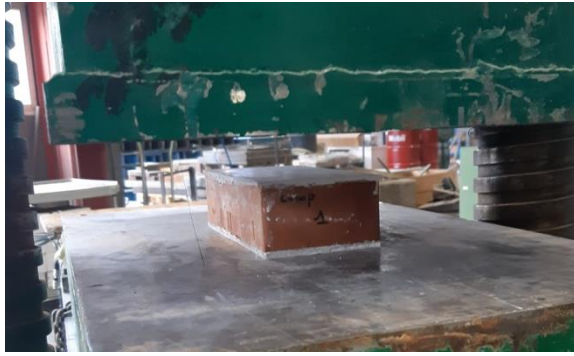
Figure 9 : Test setup of compressive strength of unit
