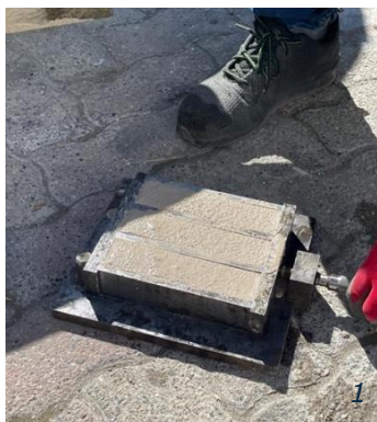
Figure 1 : Making the specimens in the mould
