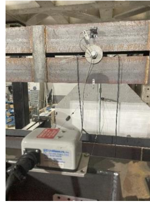
Figure 72 : Wire potentiometer on the instrumentation frame
