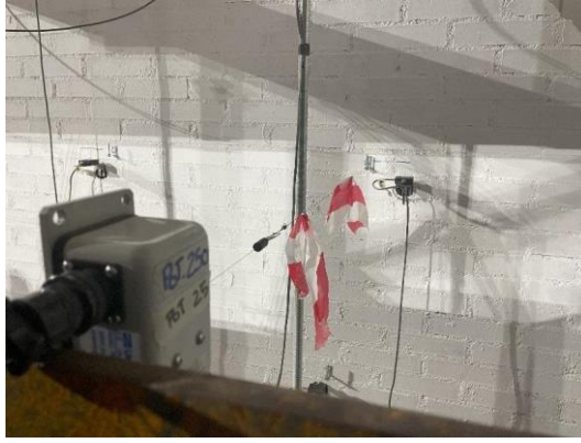
Figure 71 : Wire potentiometer measuring the relative displacement of the specimen
