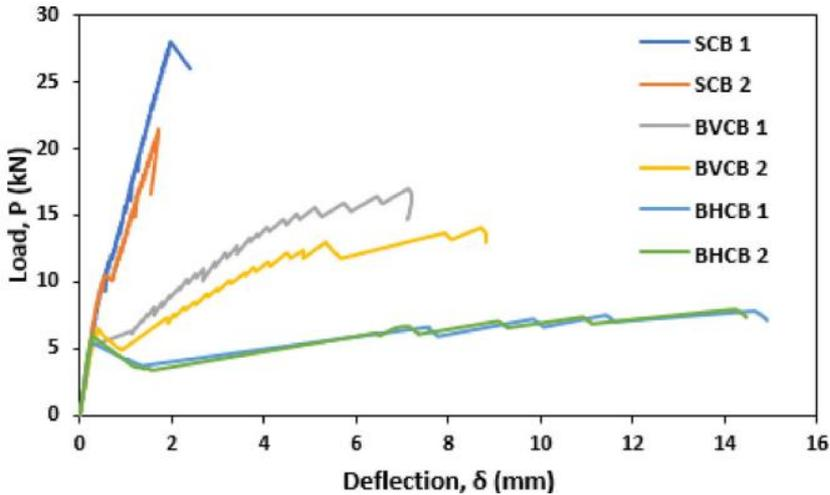
Figure 9: Results three-point bending tests [12, p. 14]
