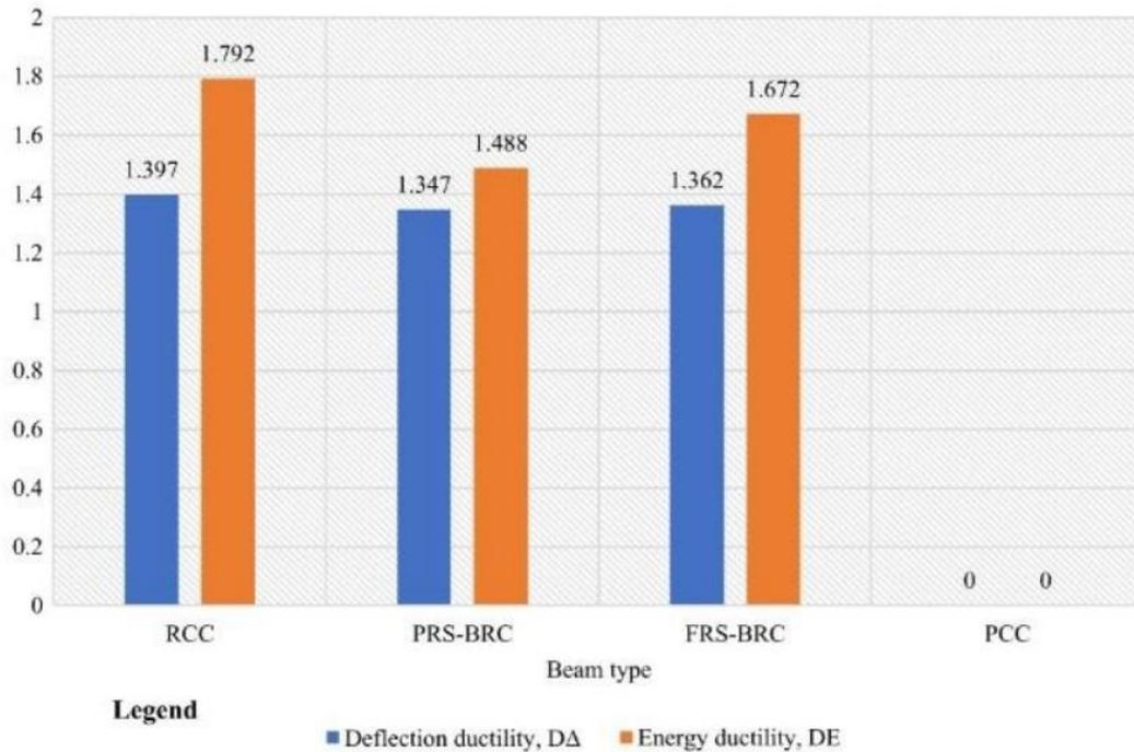
Figure 7: Ductility of the beam types [10, p. 12]
