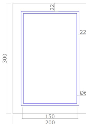
Figure 27: Cross section with transverse reinforcement
