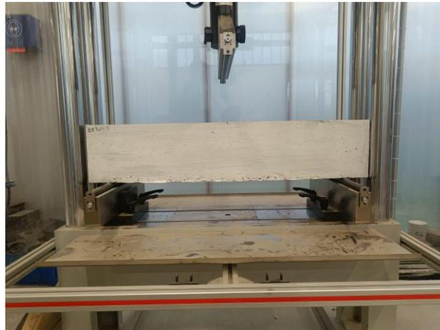
*Figure 26: Three-point bending test*
