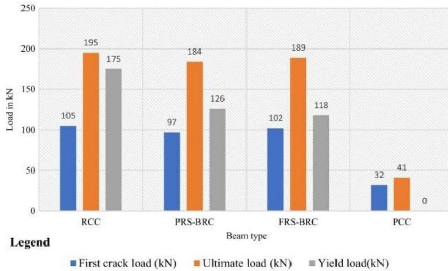
Figure 5: Maximum load per beam type [10, p. 9]
