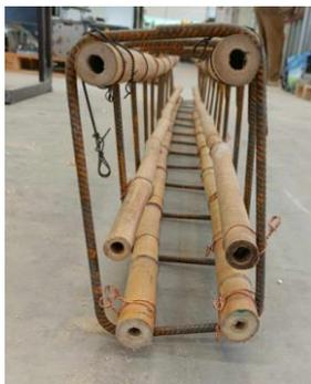
Figure 30: Reinforcement cage for BBRC
