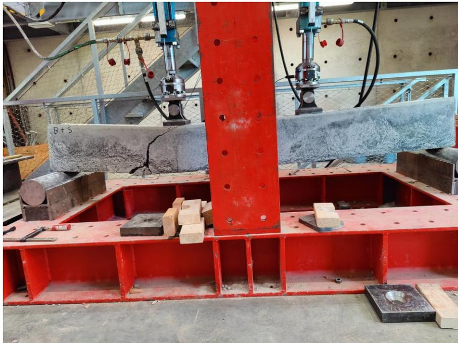
*Figure 65: Bending of the BBSRC beam*
