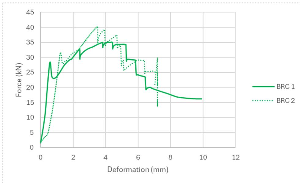
Figure 50: Force in function of deformation for BRC-beams
