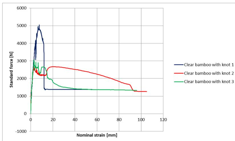
Figure 42: Clear bamboo with knot
