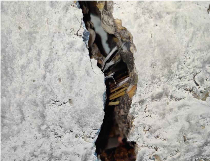
Figure 63: Close-up failure of the grooved bamboo reinforcement
