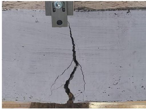
Figure 49: Cracking pattern of SRC
