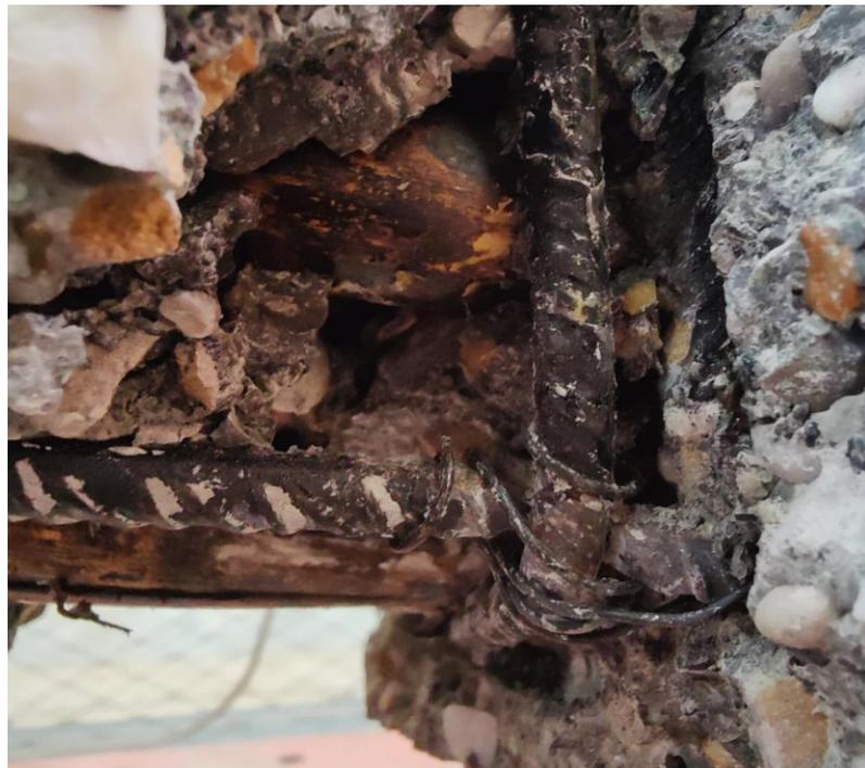
*Figure 66: Close-up failure of the bamboo and steel reinforcement*
