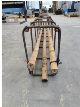
Figure 29: Reinforcement cage for BBSRC
