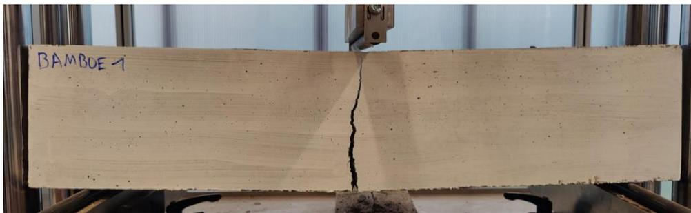
*Figure 52: Cracking pattern of BRC*
