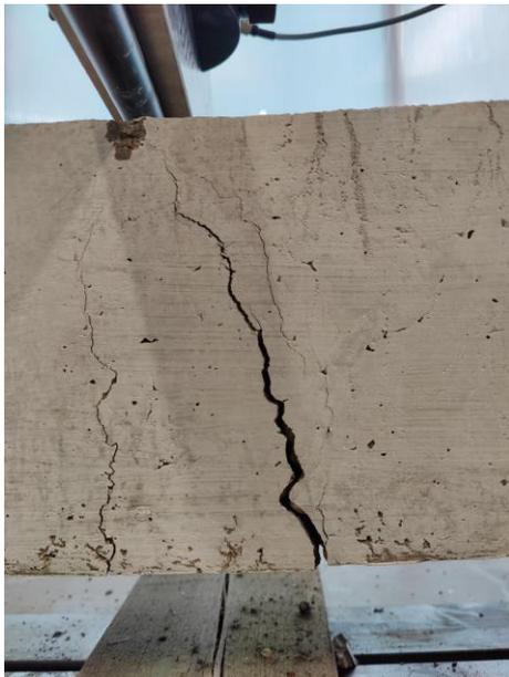
Figure 55: Cracking pattern of BBRC
