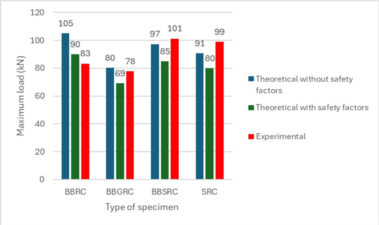
Figure 72: Comparison of the values with and without safety factors
