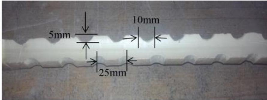
Figure 11: Bamboo strip with semi circular corrugations [13, p. 8]
