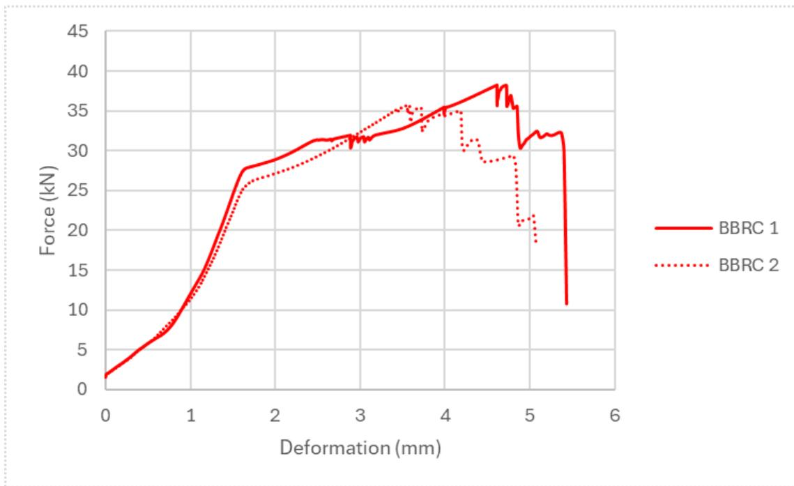
Figure 53: Force in function of deformation for BBRC-beams
