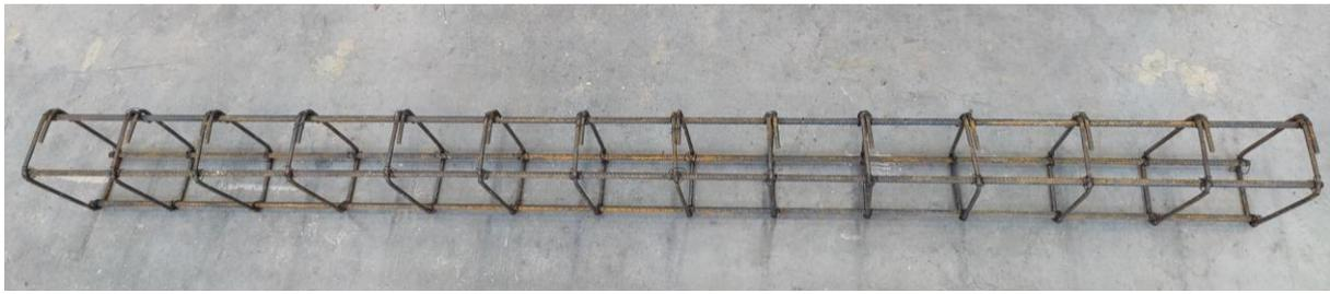
Figure 28: Reinforcement cage for SRC
