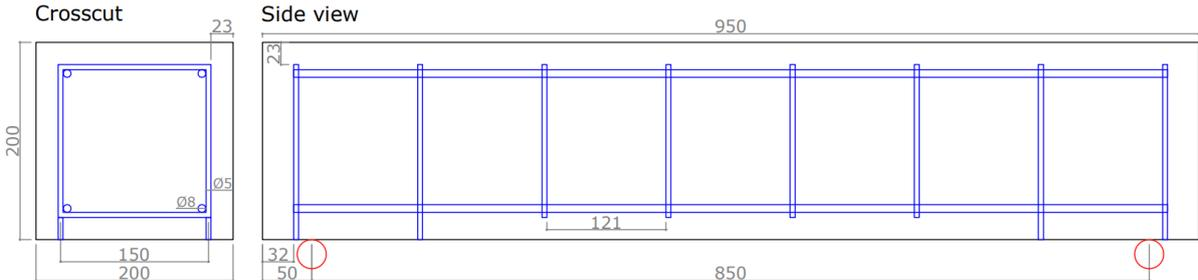
Figure 20: Dimensions of the reinforcement cage (SRC)
