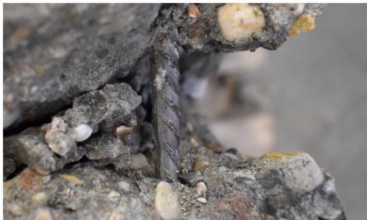
Figure 48: Necking of steel reinforcement
