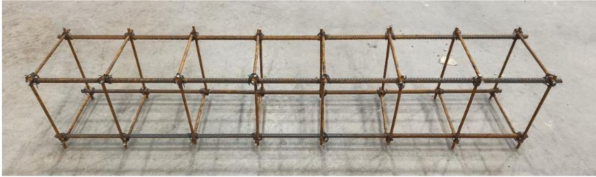
*Figure 21: Reinforcement cage for SRC*
