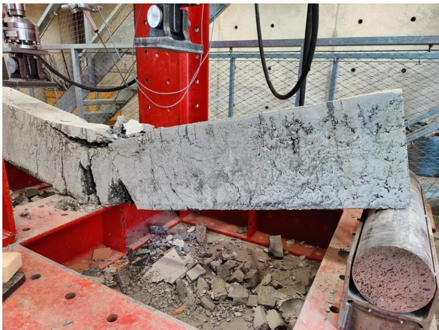
Figure 68: Bending of the SRC beam
