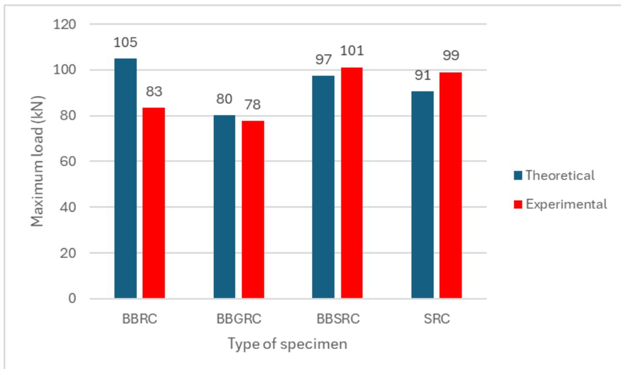
Figure 71: Maximum load theoretical vs experimental
