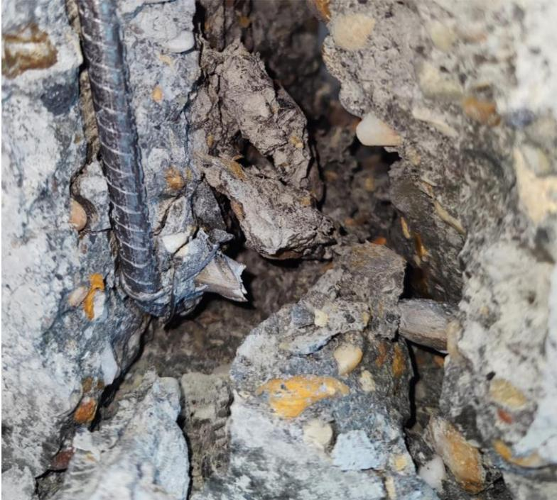
*Figure 69: Close-up necking of the steel reinforcement*
