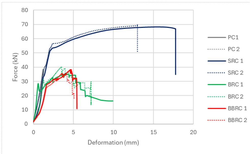
Figure 44: Force in function of deformation for all tests
