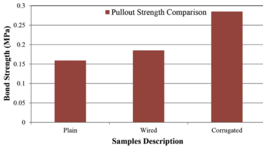
Figure 12: Bonding strengths of various types of bamboo strips [13, p. 8]
