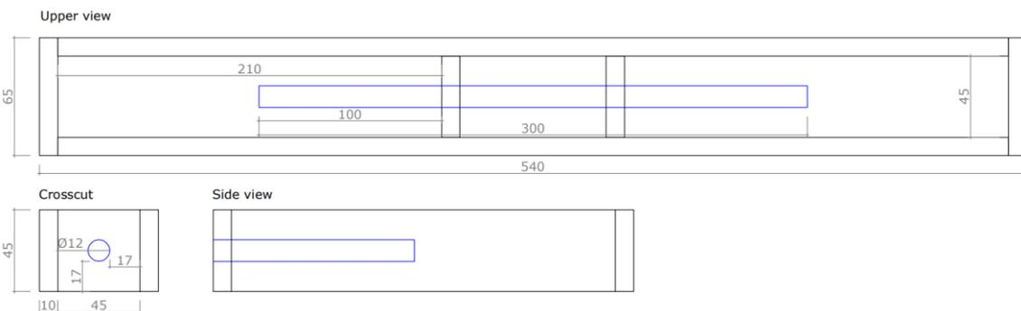
Figure 15: Pull-out test specimen dimension
