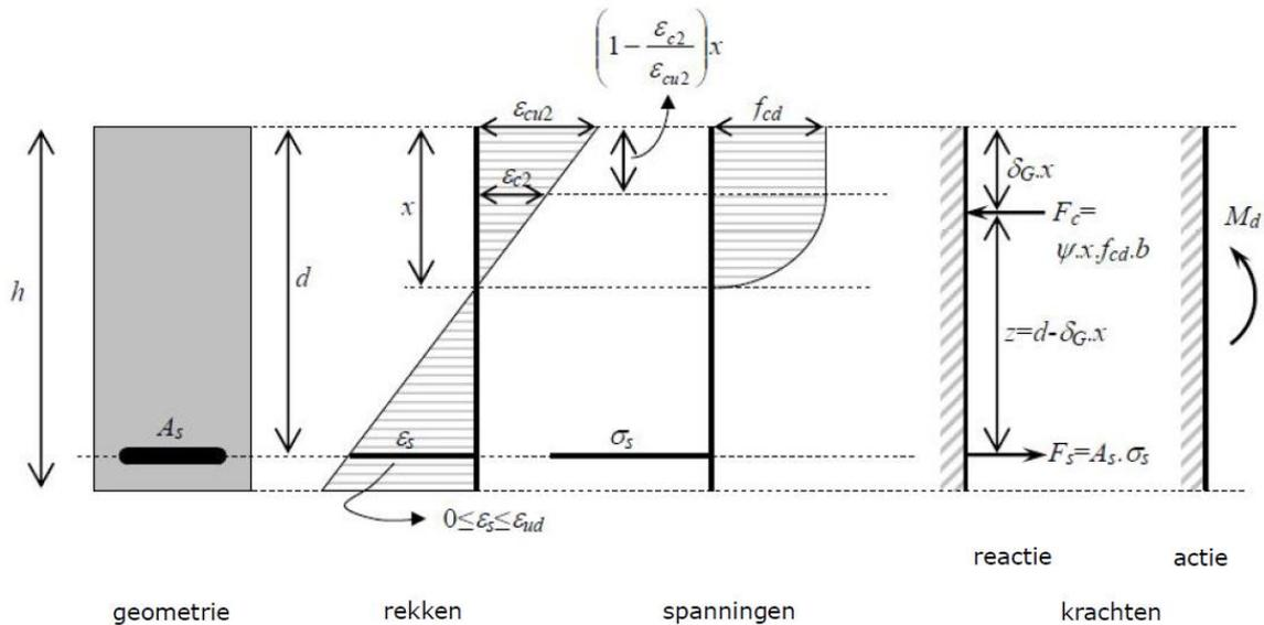
Figure 1: Strain, tension and forces diagram [2]
