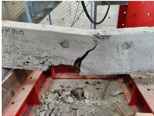
*Figure 59: Bending of the BBRC beam*
