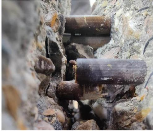
*Figure 51: Breakage of the bamboo reinforcement*
