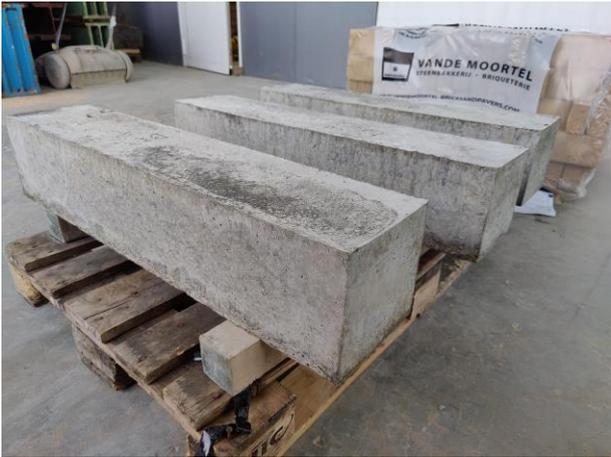
Figure 25: Demoulded small beams
