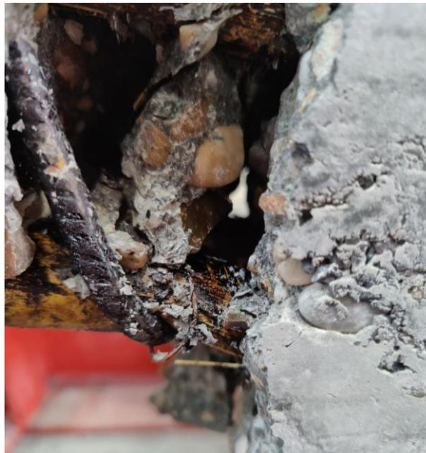
*Figure 60: Close-up failure of the bamboo reinforcement*
