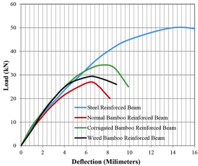
Figure 13: Load deflection curves for various concrete beams [13, p. 10]
