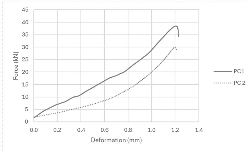
Figure 45: Force in function of deformation for PC-beams
