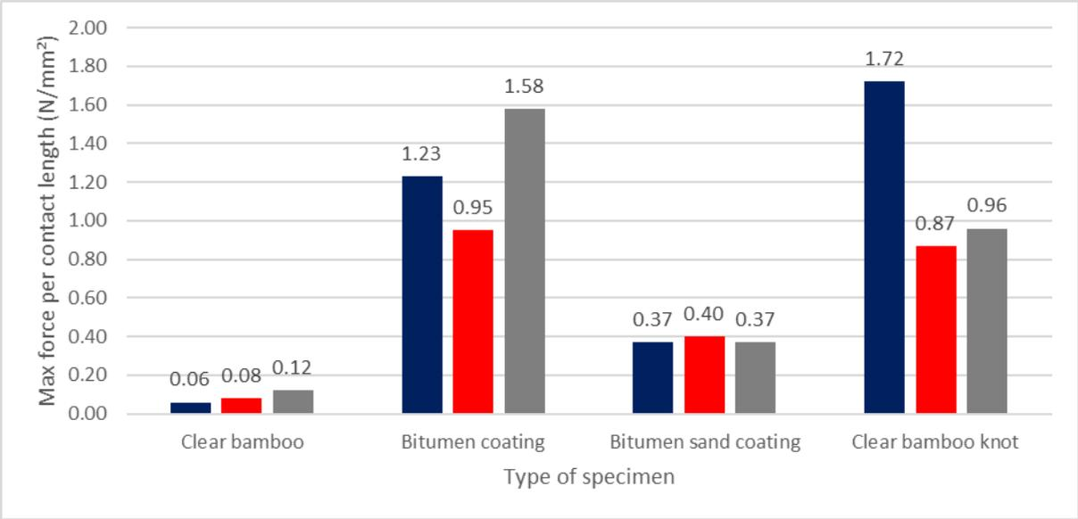
Figure 36: Results of pull-out tests
