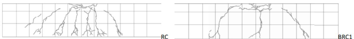
Figure 8: Cracking pattern of steel and bamboo reinforced beam [11, p. 2969]
