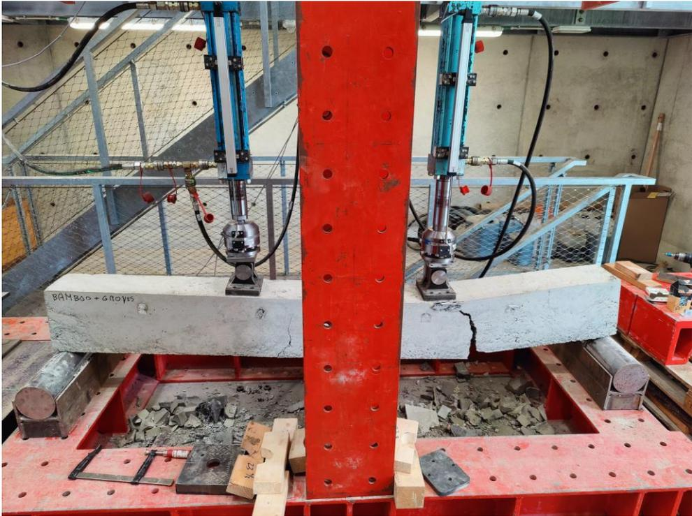
Figure 62: Bending of the BBGRC beam
