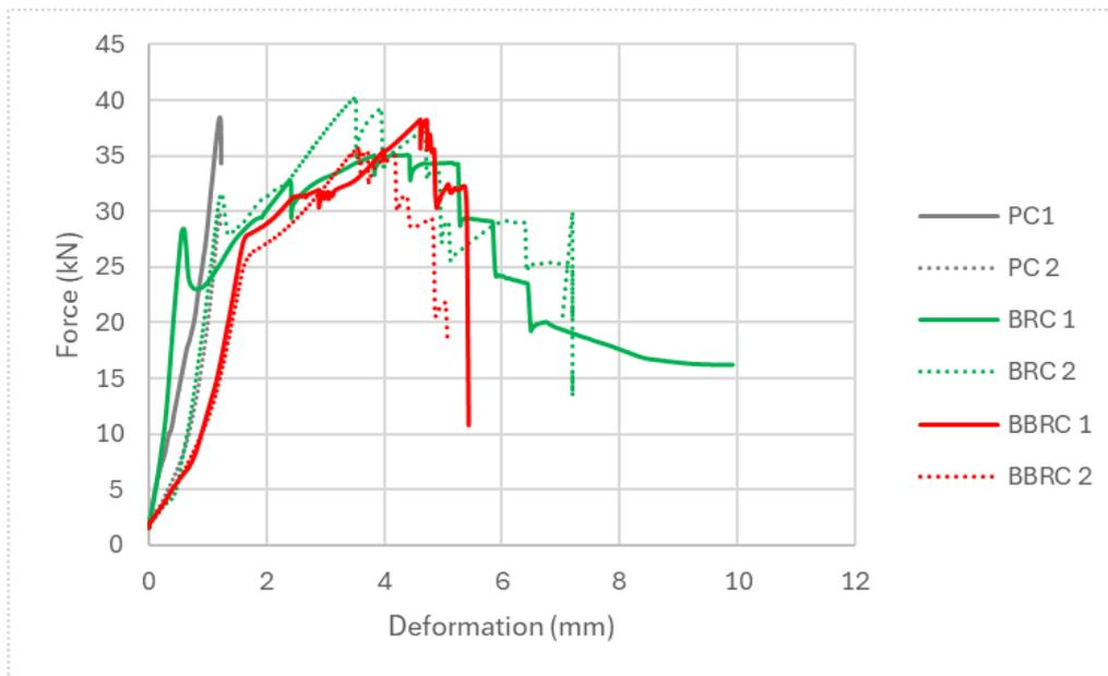
Figure 57: PC, BRC and BBRC beams compared
