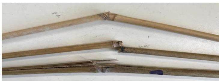
*Figure 4: Breaking of bamboo with a knot after bending test [3, p. 81]*
