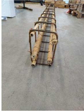
*Figure 31: Reinforcement cage for BBGRC*
