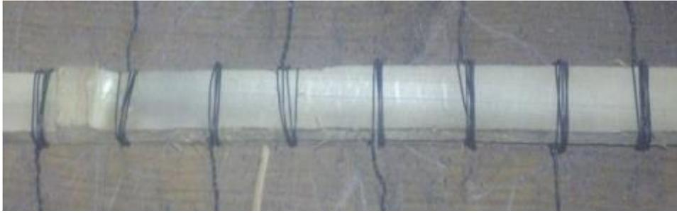
Figure 10: Bamboo strip with wire wrappings [13, p. 8]
