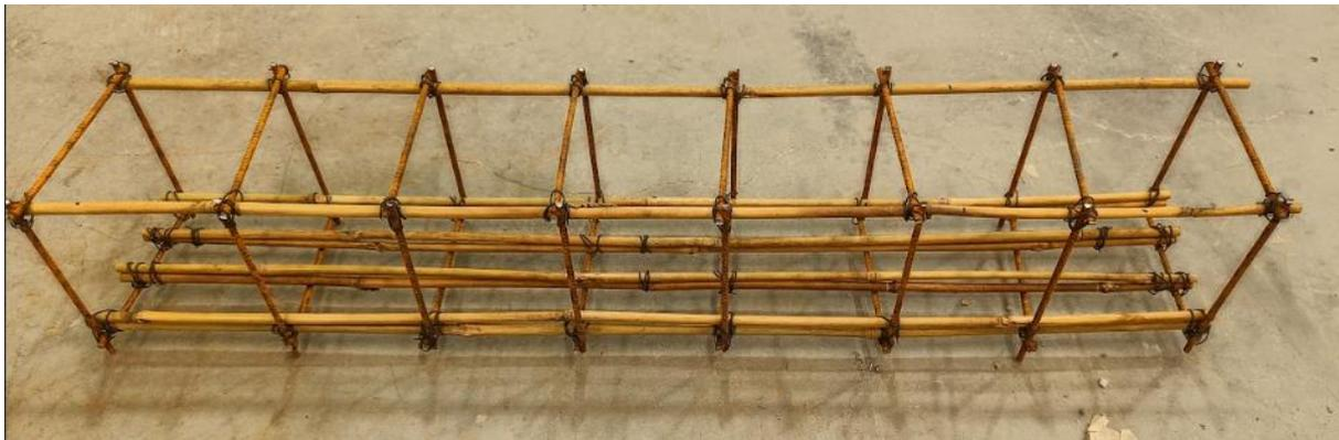
*Figure 22: Reinforcement cage for BRC*
