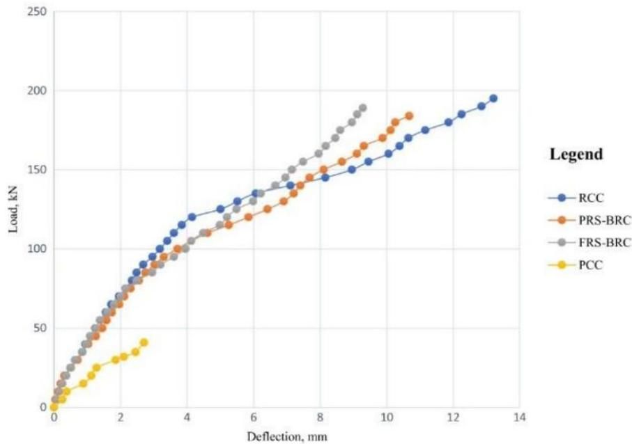
Figure 6: Load in function of deflection [10, p. 10]
