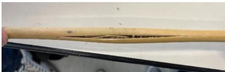
*Figure 3: Splitting of bamboo without a knot after bending test [3, p. 80]*
