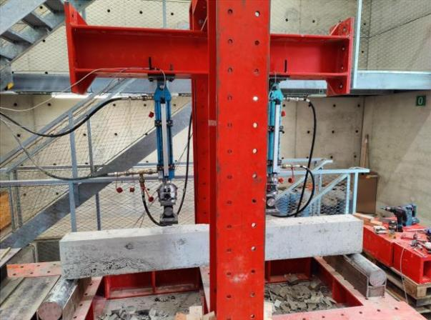
Figure 34: Four-point bending test
