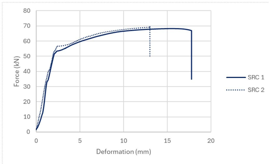
Figure 47: Force in function of deformation for SRC-beams
