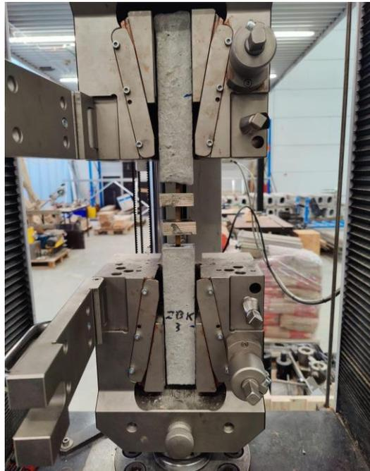
*Figure 19: Pull-out test setup*
