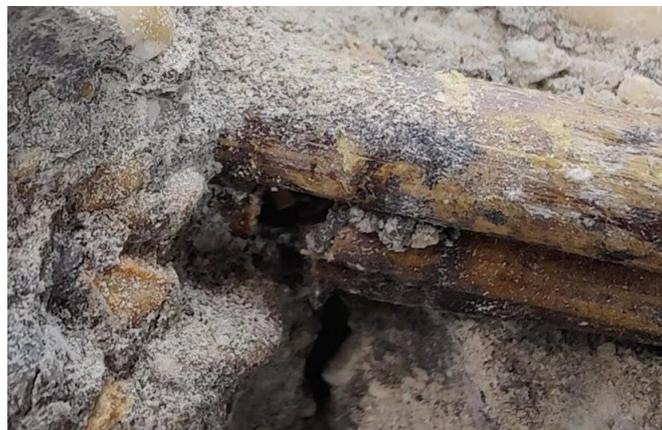
Figure 54: Breakage of the bamboo with bitumen reinforcement
