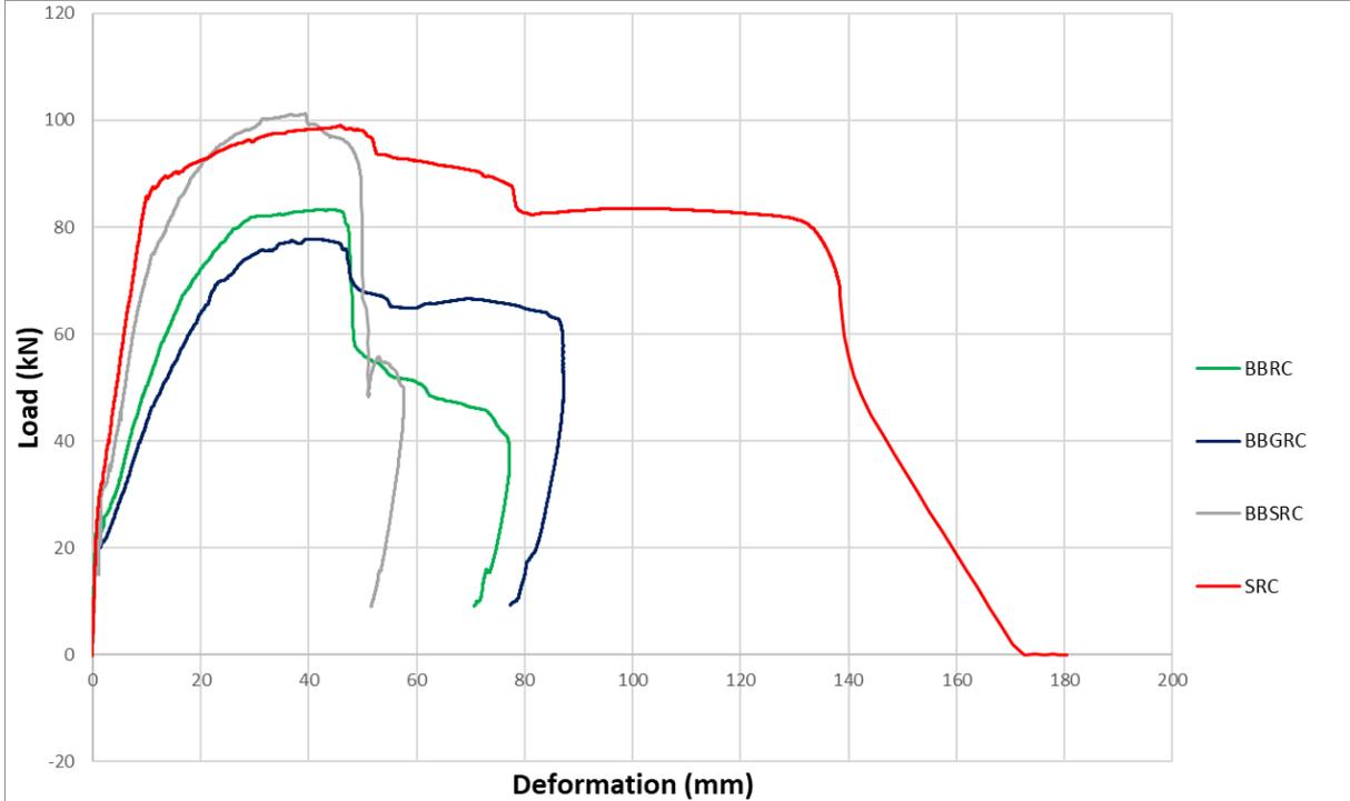
Figure 70: Total load for each type of reinforcement
