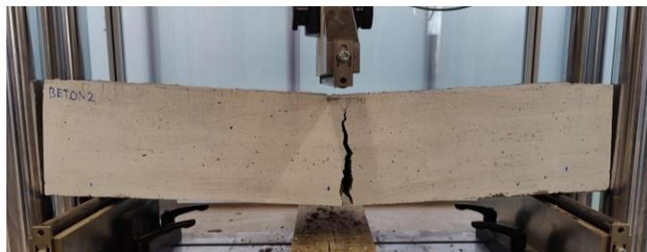
Figure 46: Cracking pattern of PC
