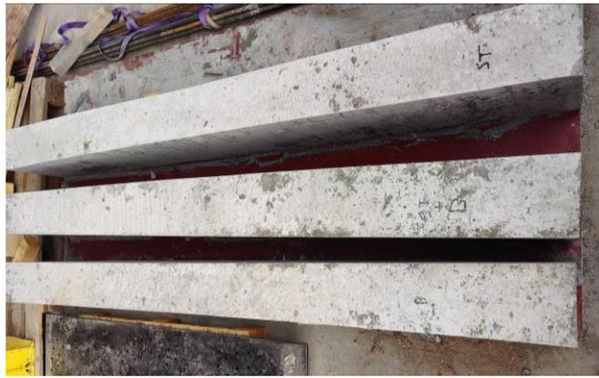
*Figure 33: Demoulded large beams*
