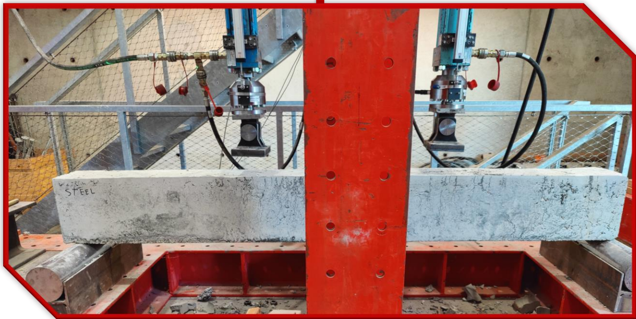
Figure 3: Four-point bending test
