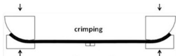
Figuur 2.6: Pre bending [15]
