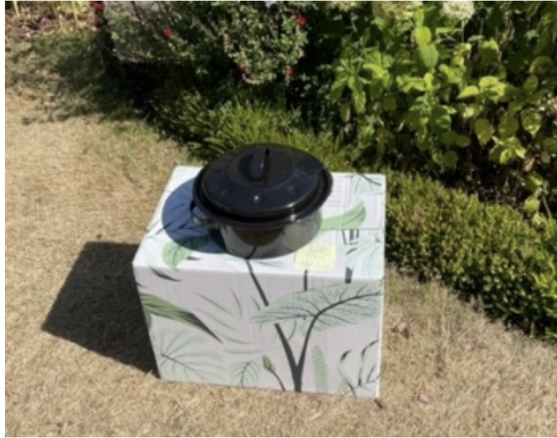
Figure 1: Picture showing a black port, labelled as OnlyPot which is positioned outdoors to receive direct sunlight without a plastic bag around the pot. The OnlyPot is not among the locally made prototypes was merely used for comparison purposes.
