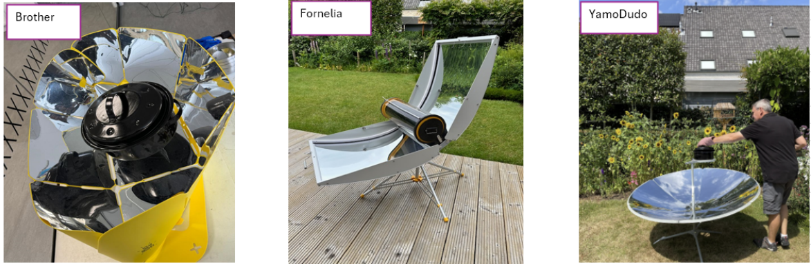
Figure 4: Picture showing the commercial available cookers included in the performance evaluation (left) Brother, (middle) Fornelia, and (right) YamoDudo
