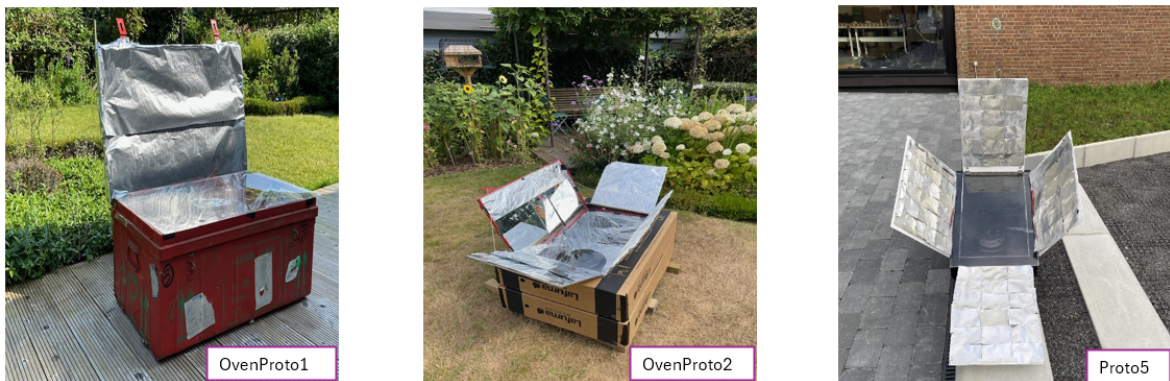
Figure 3: Picture showing locally made oven prototypes (left) OvenProto1 contains one reflective panel covered with aluminum foil, (middle) OvenProto2 contains 4 reflective panels covered with aluminum foil and (right) Proto5 contain 4 reflective panels that are covered with soda cans. The prototypes are covered with plastic glass on top that accounts for the plastic bag effect.
