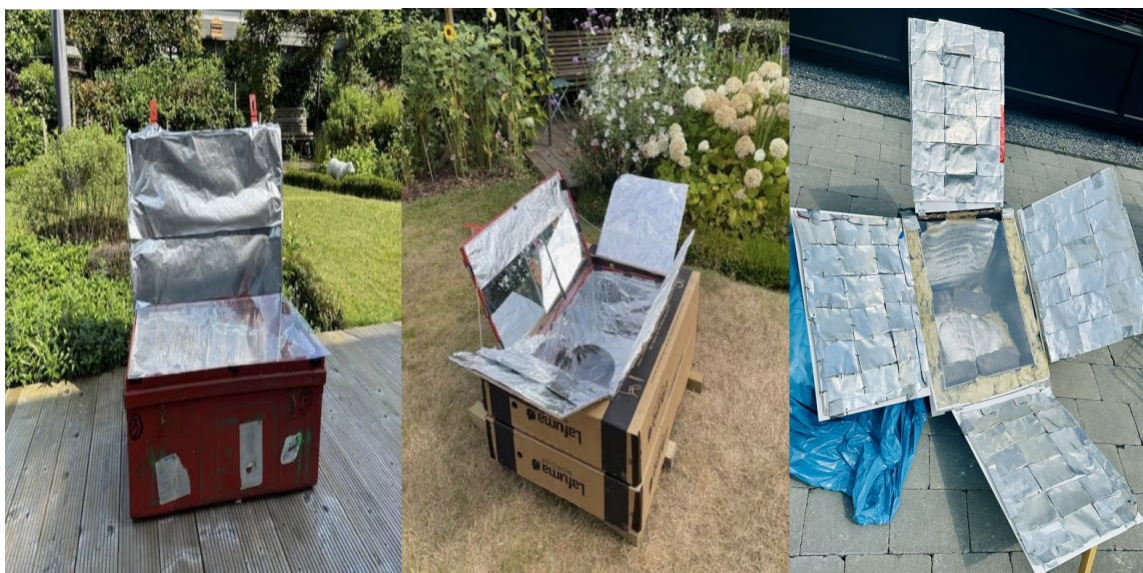
Figure 2: Oven_Prototype 1 (Left), Oven_Prototype 2 (middle), and Prototype 5 (right); all covered with plastic glass on top.
