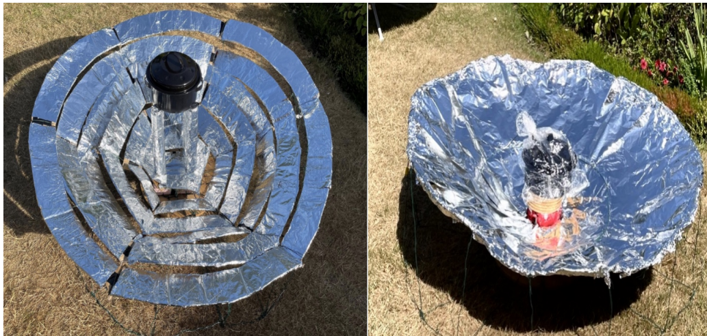
Figure 3: Prototype 2 with the pot not covered by a plastic bag (left), and Prototype 2/3 with the pot covered by a plastic bag (right).
