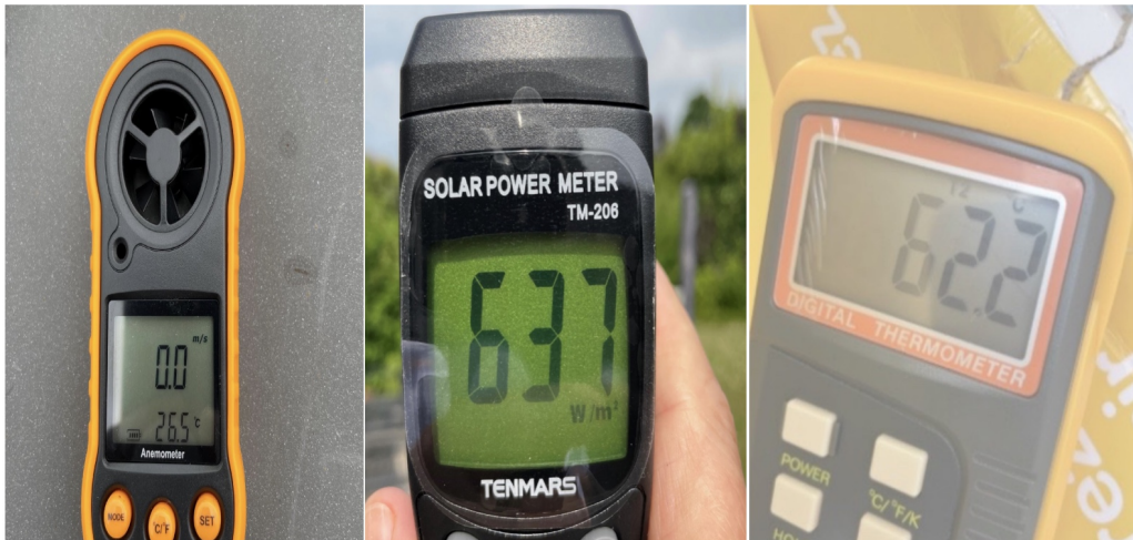
Figure 5: An anemometer (left), Pyranometer (middle), and Digital Thermometer (right) with readings of wind speed and ambient temperature, solar irradiance, and water temperature respectively.
