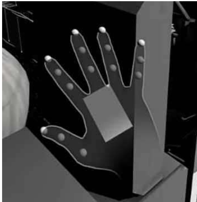
Figure 3.10: The sphere and box collider for the right hand when the mesh renderers are enabled.
