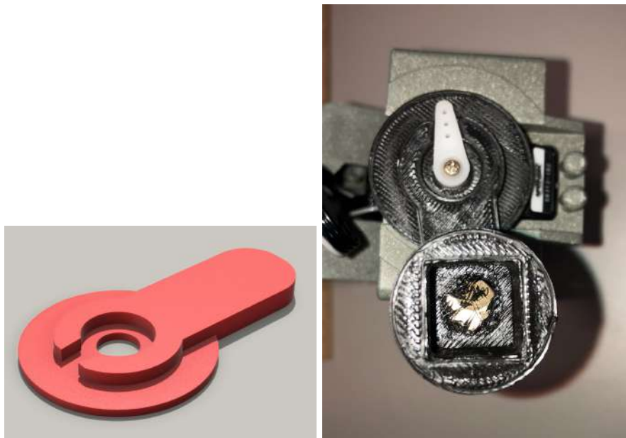
(a) The 3D-printed grip latch, which rotated according to the wrist-roll servomotor, could be modified to accommodate additional attachments. (b) The top part of the image shows the grip latch, including the screw and plastic insert. The bottom part displays a female magnet holder with a magnet inside.
