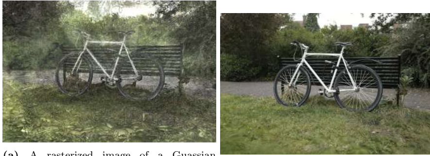
(a) A rasterized image of a Gaussian Splatting representation where every gaussian of the bicycle is rasterized as fully opaque[HS23]. (b) The normal Gaussian Splatting method where the bicycle image is rasterized with non opaque Gaussians[HS23].
