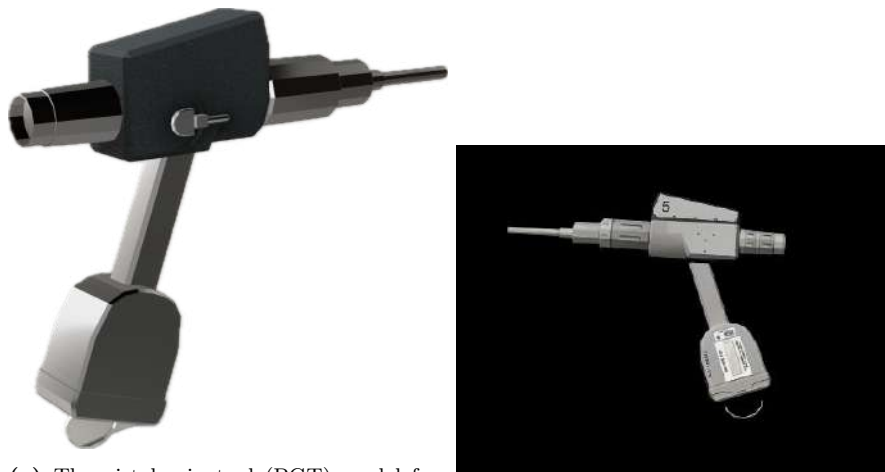
(a) The pistol grip tool (PGT) model features custom textures and can function as a (b) The pistol grip tool (PGT) model with screw with adjustable dynamic torque [GN]. original textures[GN].
