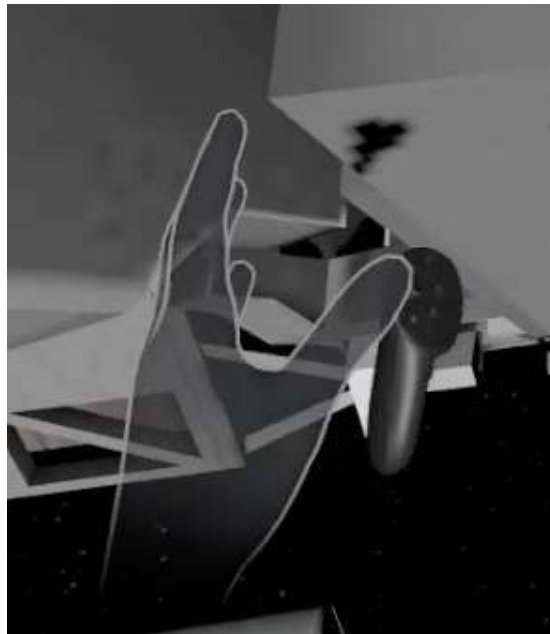
Figure 3.12: The left hand and the left controller are always simultaneously tracked and always shown.
