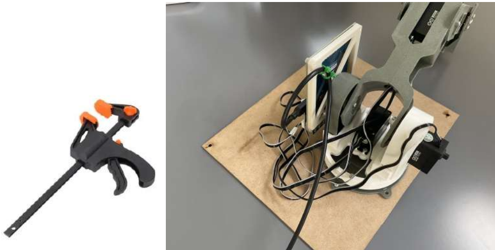
(a) The grip ratchet clamp used to keep the robot arm in place on the table. (b) The zip tie brace alleviating the stress on the Micro-USB port on the board by transferring the stress to the mounting port underneath the Arduino Board.
