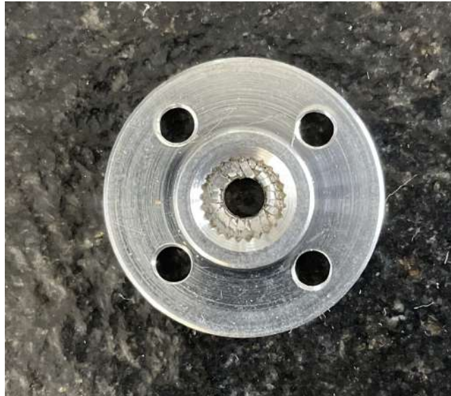
(c) The replacement metal horn.
