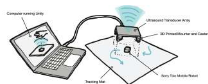
(f) System Design to enable 2D translations of ultra-sound transducers using Sony Toio tabletop robots[FFS22].
