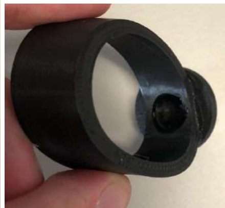
(d) The controller mount slanted on its side to see the magnet hole for the controller mount and the male magnet holder.
