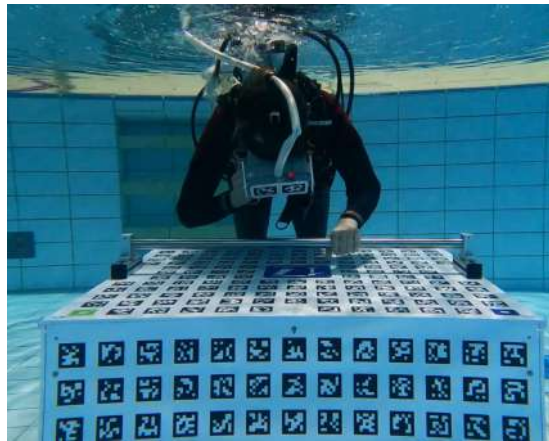
Figure 2.13: VR headset integrated with a full-face diving mask, featuring head tracking via an underwater camera system and a physical handrail replicated in VR[Age23].
