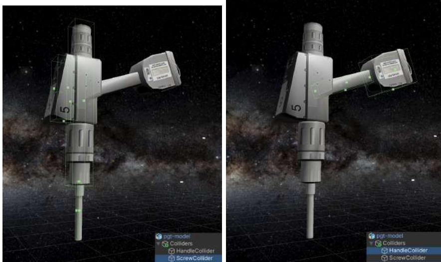
(a) The box colliders associated with the screw of the PGT tool.
