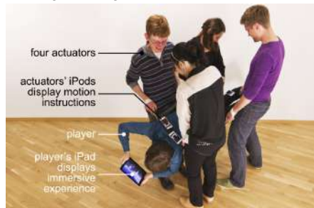
(c) Haptic turk allows producing motion experiences anywhere anytime. Here, the suspended player is enjoying an immersive hang gliding game. The four actuators create just the right physical motion to fill in the player's experience[Che+14].
