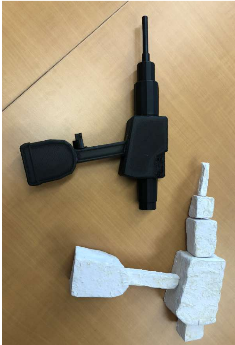
Figure 4.12: The 3D printed PGT at the top left and the styrofoam PGT at the bottom right. The 3D printed PGT includes a slide and lock magnet mechanism for easy lateral magnet removal.
