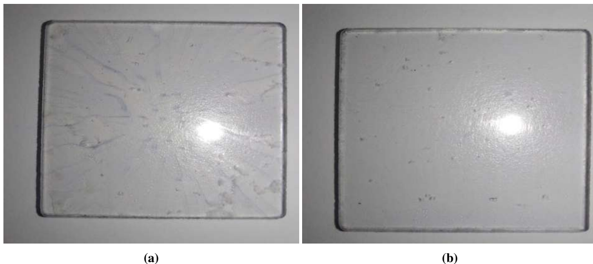
Figure 8: Spin coating of PEDOT:PSS mixed with (a) DMSO resulted in rough film morphology, and (b) glycerol resulted in smooth film morphology.
