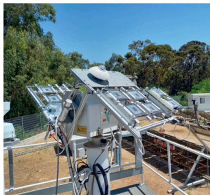
Figure 3. Perovskite mini-modules located outdoors and tested side by side.
