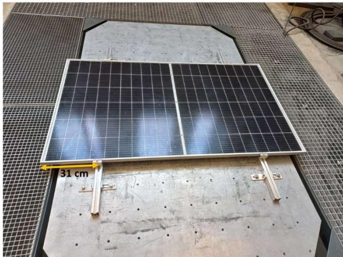
*Figure 1. PV module fixed on the vibration table with aluminum profiles-supports. The exact position of the clamps is indicated.*
