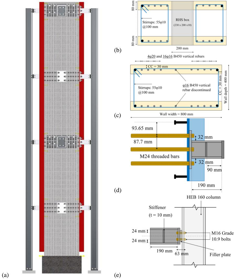
**Fig. 2.** (a) Overview of the designed specimen, (b)-(c) sectional view of the wall cross-section with and without the RHS box, (d) link-to-wall connection and (e) link-to-column connection.
