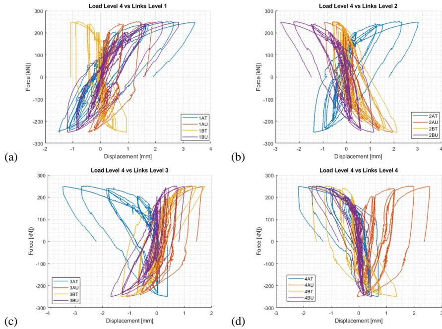
**Fig. 7.** Deformation in the links corresponding to the load applied at the top of the HCW, (a) 1<sup>st</sup> storey, (b) 2<sup>nd</sup> storey, (c) 3<sup>rd</sup> storey and (d) 4<sup>th</sup> storey
