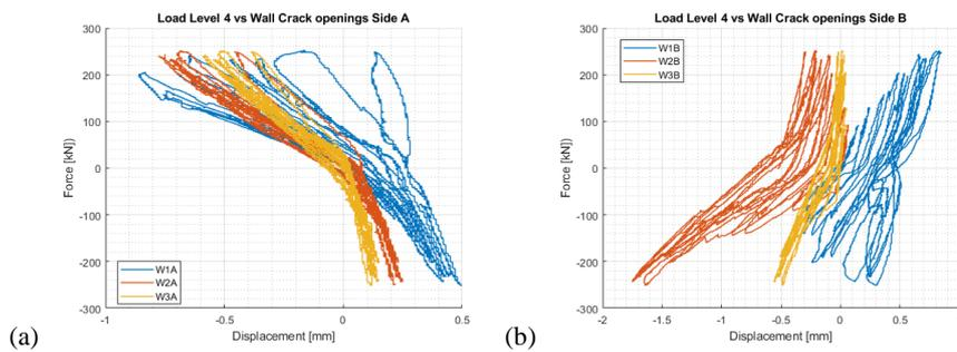
**Fig. 8** Evolution of cracks at the ground storey of the wall with respect to the load applied at the top of the HCW, (a) Side A and (b) Side B
