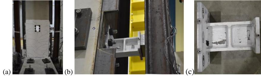
**Fig. 9.** Images showing the final state of (a) the bottom part of the RC wall and (b)-(c) a link
