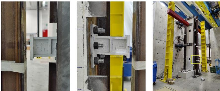
**Fig. 10.** Removing a damaged link at the ground storey level of the HCW
