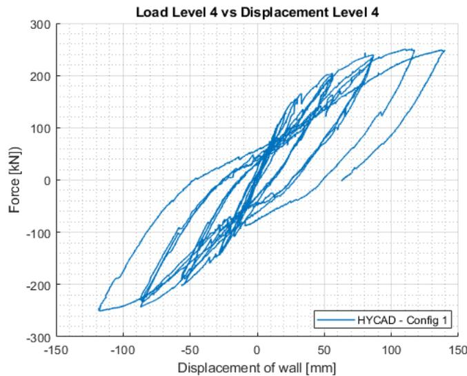
**Fig. 6.** Global force-displacement curve obtained from the top of the HCW
