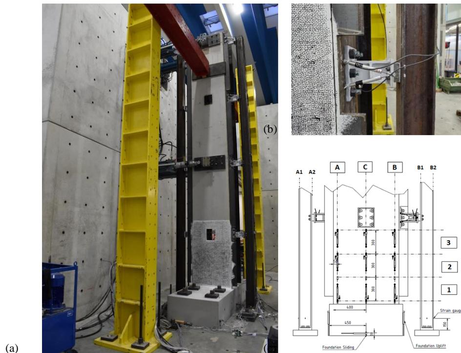
**Fig. 3.** (a) Real-life test set-up with instrumentation on (b) links and (c) wall
