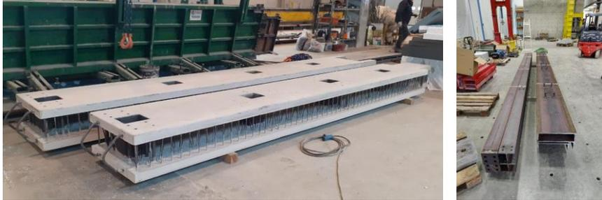
**Fig. 4.** Prefabricated DS walls and steel parts
