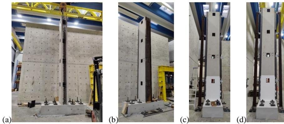
**Fig. 5.** (a) First stage and (b) second stage of casting, (c) & (d) attaching links and columns
