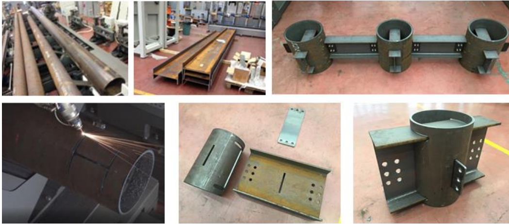
Fig. 1. Laser cutting techniques, machine and approach to develop the LASTEICON and LASTTS joints (2)
