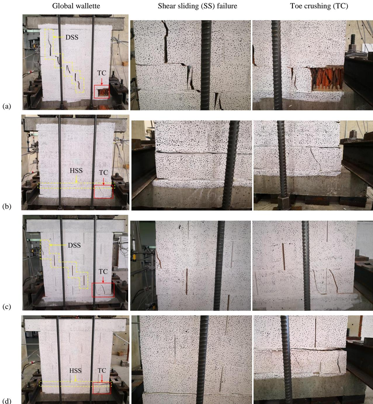
**Figure 17.** Ultimate failure modes of the wallettes: (a) TTN1 – Diagonal shear sliding (DSS) with toe crushing (TC), (b) TAND2 – Horizontal shear sliding (HSS) with toe crushing (TC), (c) PPG2 – Diagonal shear sliding (DSS) with toe crushing (TC) and (d) PAND3 – Horizontal shear sliding (HSS) with toe crushing (TC).
