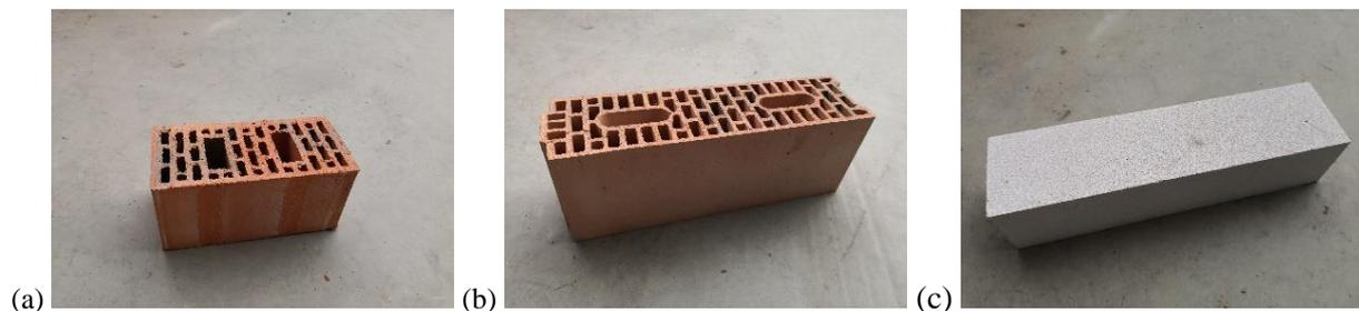
**Figure 2.** Masonry units used in experiments: (a) clay brick for GPM, (b) clay brick for TLM, (c) AAC block.
