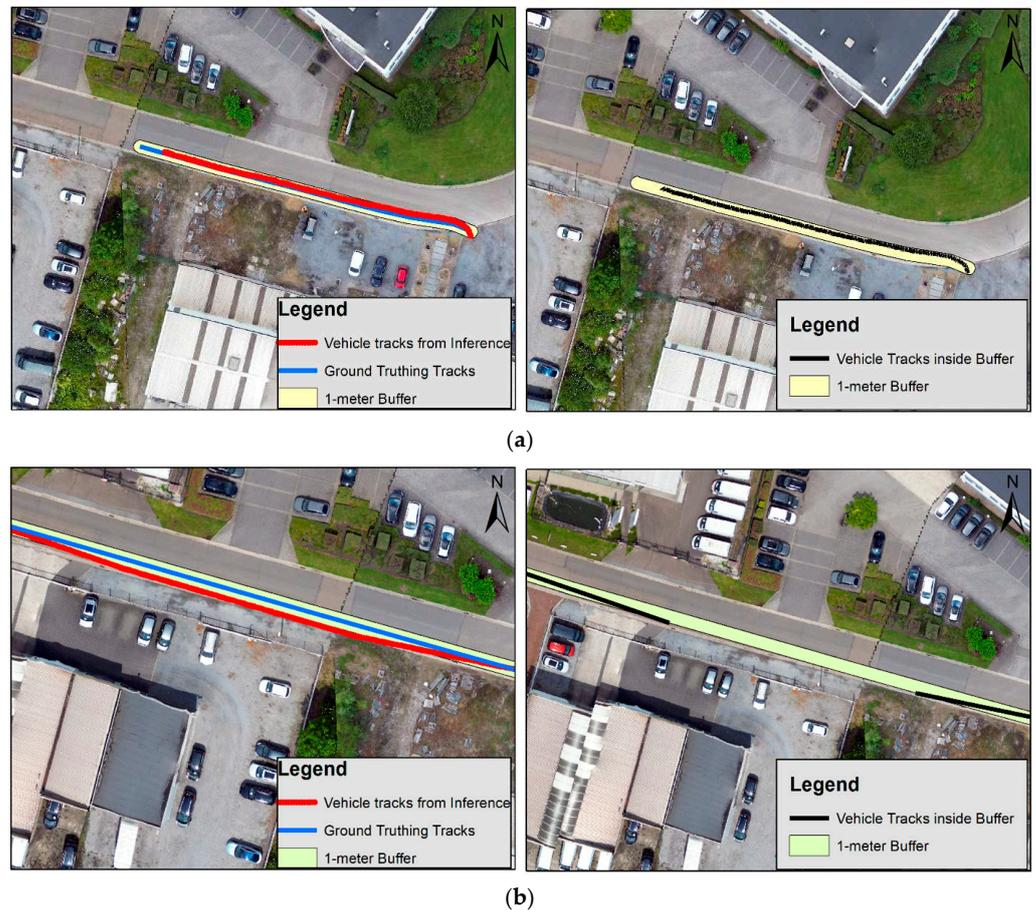
**Figure 8.** The method used for determining the positional accuracies of vehicle tracks on (a) tracks from stationary drone footage and (b) tracks from moving drone footage.
