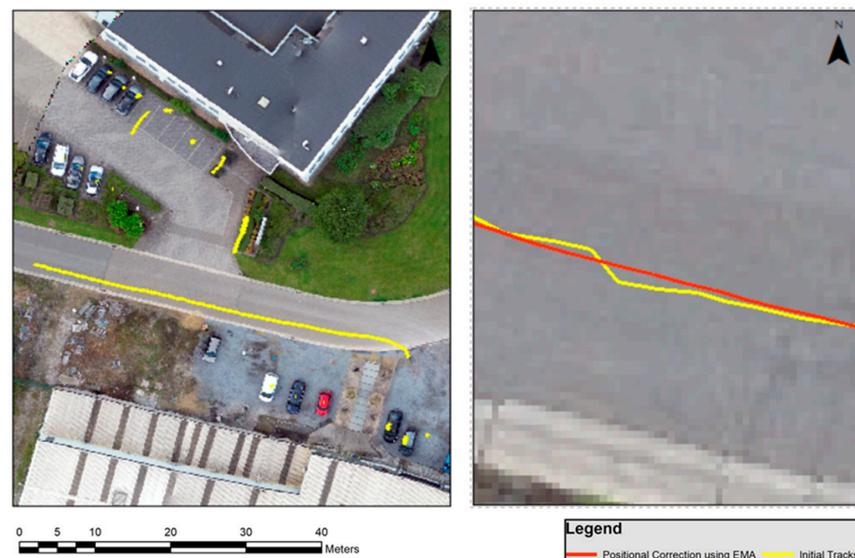
**Figure 4.** The mapped vehicle trajectories before and after EMA application.
