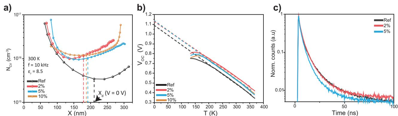
**Figure 2.** a) Carrier density profiles extracted by C-V analysis. b) Plots of  $V_{OC}$  versus temperature ( $V_{OC}$ - $T$ ) and linear fits of the recombination  $E_a$  of the devices. c) TRPL decay for the Ref and low Li content devices.
