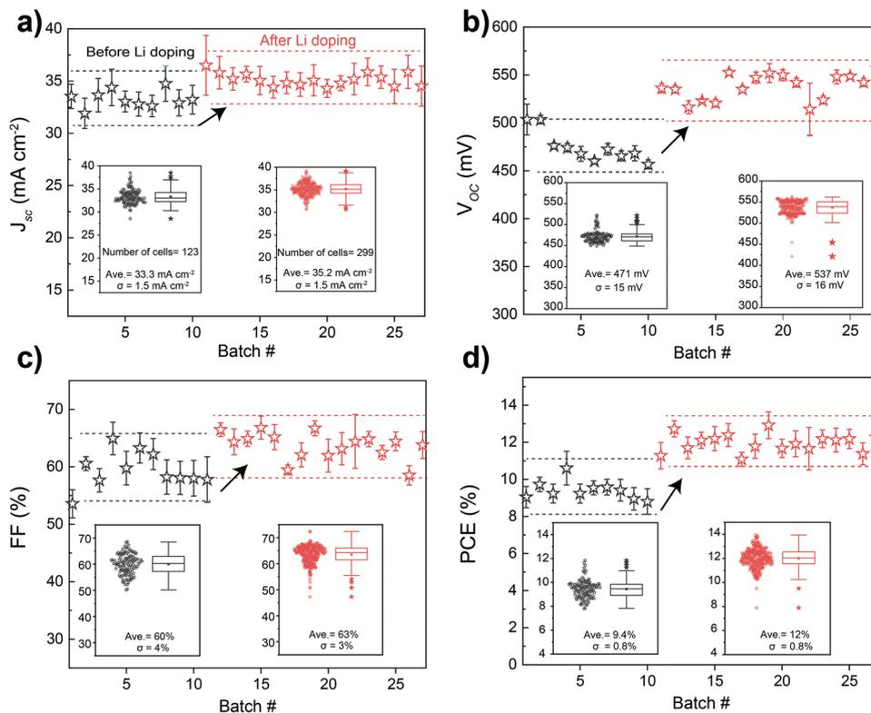
**Figure 7.** PV parameters of different batches of device before and after the implementation of optimal Li doping conditions: a)  $J_{SC}$ , b)  $V_{OC}$ , c) FF, and d) PCE. Dashed lines are included as visual aid.
