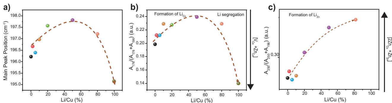
**Figure 4.** a) Plot of the ACZTSSe main peak position in Raman spectra as a function of Li content. b) Plot of the area ratio of the 176 cm<sup>-1</sup> peak to the main peak. c) Plot of the area ratio of the 250 cm<sup>-1</sup> peak to the main peak.
