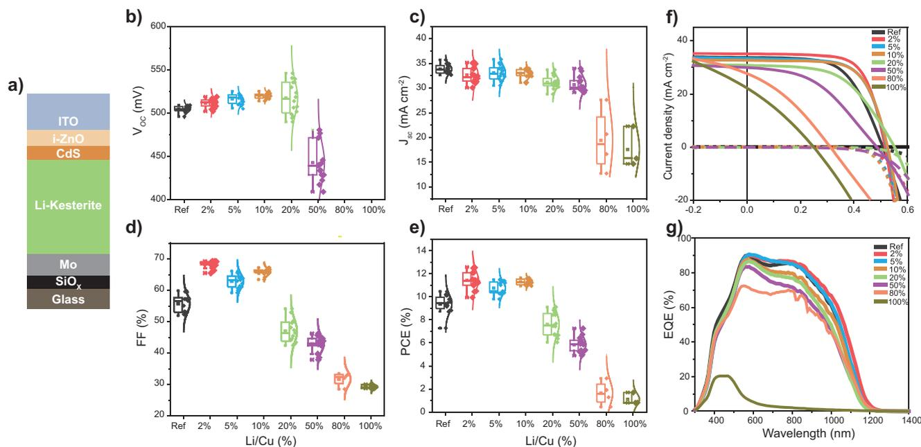
**Figure 1.** a) Schematic structure of the kesterite device based on a soda lime glass substrate with a SiO<sub>x</sub> Na barrier layer. b–e) Statistical distribution of the photovoltaic parameters for devices with varying Li content. f) Representative illuminated and dark  $J$ - $V$  curves of the devices for varying Li content. g) EQE spectra of the device for varying Li content.
