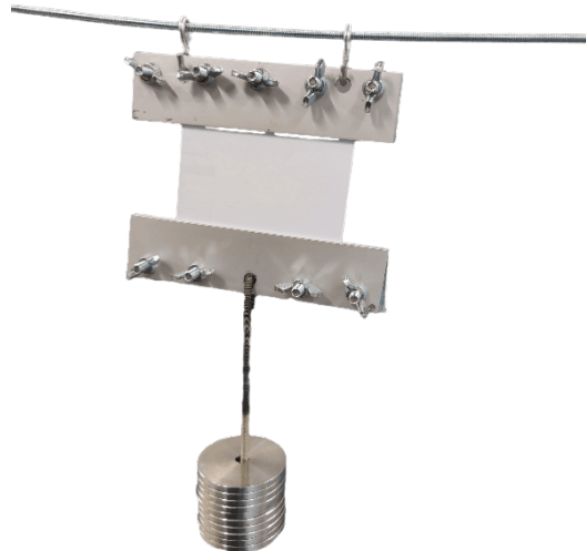
Figure 1: Self-made metal construction to stretch multilayer films using gravity in an oven.
