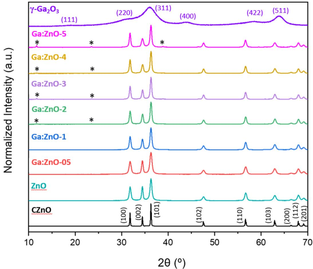
**Figure 2.** Powder X-ray diffraction patterns of commercial ZnO, and as-synthesized undoped ZnO, Ga-doped ZnO with variant gallium content and pure  $\gamma$ -gallium oxide nanomaterials. Commercial zinc oxide is used as reference material for the samples containing zinc oxide. Symbol: \*-corresponds to the secondary phase Zinc gallium carbonate LDH.
