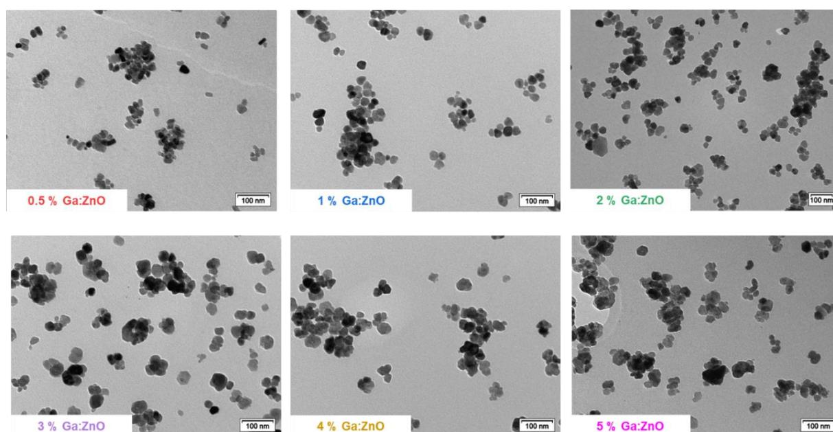
**Figure 1.** TEM micrographs of the Ga-doped ZnO from Ga:ZnO-05 to Ga:ZnO-5 as-synthesized materials.
