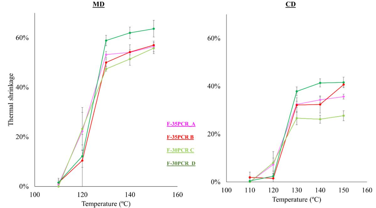
Figure 6: Thermal shrinkage of films in machine direction (MD, left) and cross direction (CD, right).
