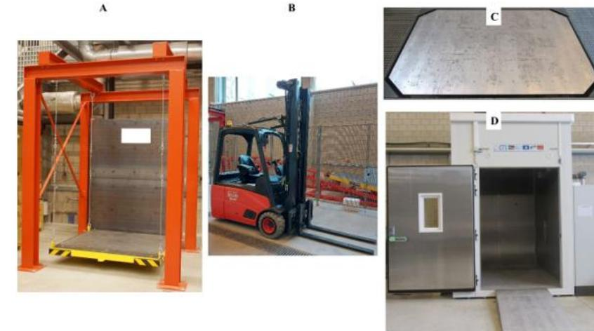
Figure 2: Transport simulation equipment used in this study. (A) swing device to simulate horizontal collisions; (B) forklift for pallet transport; (C) vibration table; (D) walk-in climate chamber.
