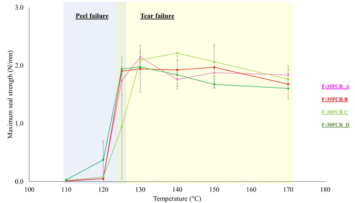
Figure 5: Evolution of maximum seal strength and failure mechanisms (peel, tear) of the inner side of films as a function of bar temperature.
