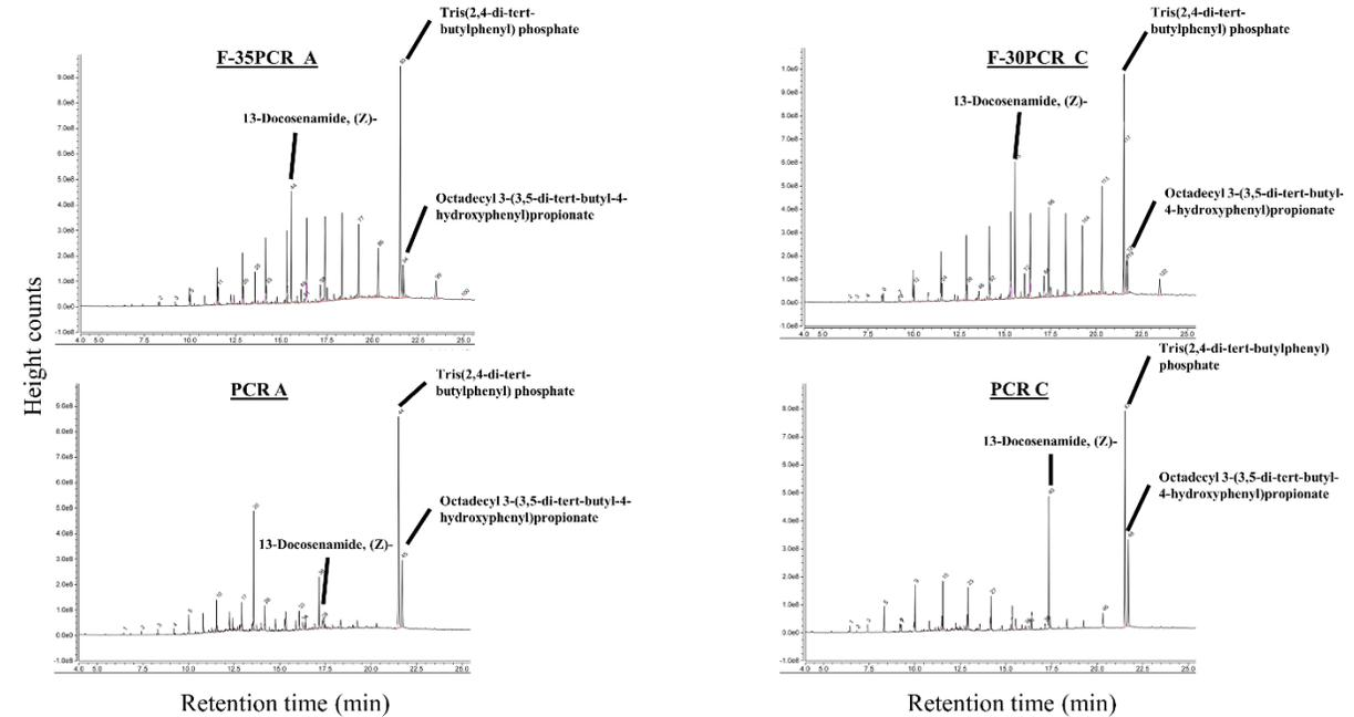
Figure 4: Mass spectra of F-35PCR\_A and F-30PCR\_C, alongside the spectra of their respective PCR granulates.
