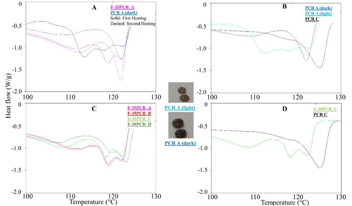
Figure 3: DSC thermograms: (A) two heating cycles of F-35PCR and PCR A; (B) first heating of two granulate types, with PCR A split by colour (dark and light); (C) first heating of four films compared; (D) first heating of F30PCR A vs. PCR 2.
