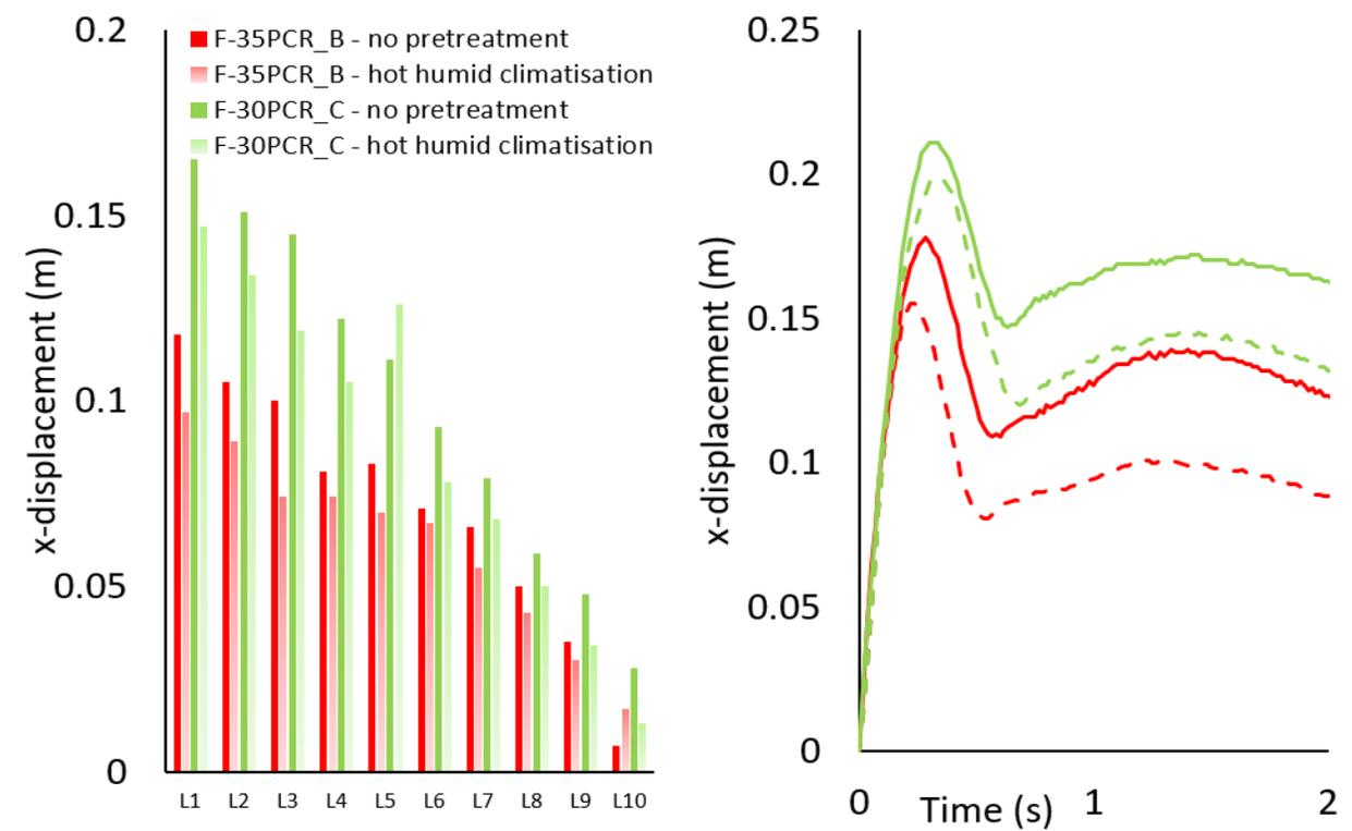
Figure 7: Horizontal displacements of the 10 brick layers after the swing test (left), with L1 as the top layer and L10 as the bottom, and during the swing test (right, only the top layer), caused by tilting.
