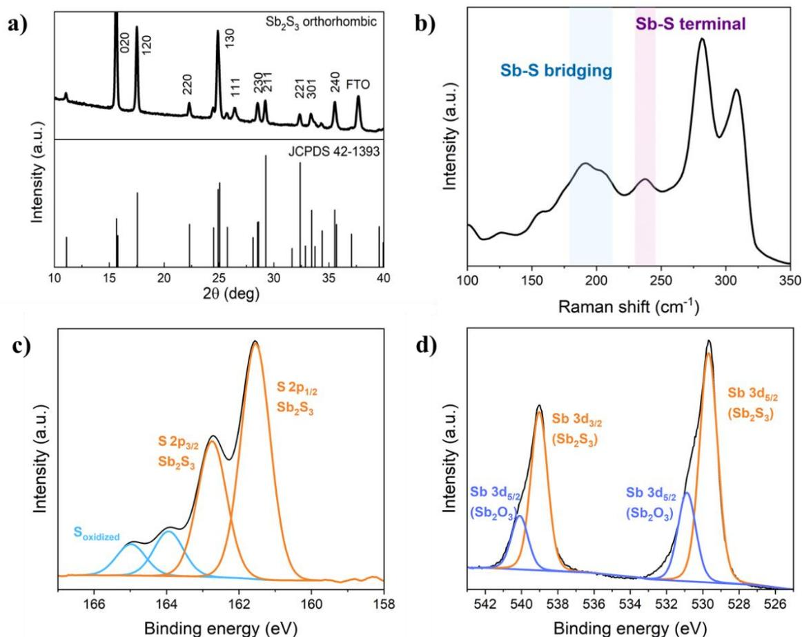
**Figure 1.** a) XRD patterns, b) Raman spectra, and c) S 2p d) Sb 3d XPS high resolution spectra of Sb<sub>2</sub>S<sub>3</sub> thin films prepared by thermal evaporation on FTO coated glass.
