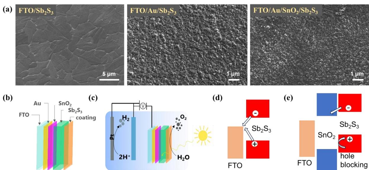
**Figure 4.** **a)** Surface SEM images of thermally evaporated Sb<sub>2</sub>S<sub>3</sub> on different substrates **b)** Schematics of photoanode architecture **c)** Schematics of device working principles for PEC water oxidation. Schematics of activity of the Sb<sub>2</sub>S<sub>3</sub>-based photoanode **d)** without and **e)** with SnO<sub>2</sub> as ETL and holes block layer.
