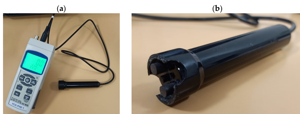
Figure 2. (a) Conductivity meter PCE-PHD 1 from PCE Instruments with (b) modified conductivity sensor.
