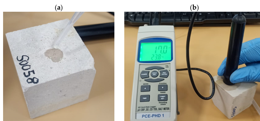
Figure 3. Conductivity measurement on Silos stone. (a) Additions of a drop distilled water; (b) measurement.
