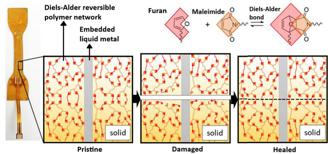
Fig. 1. Schematic of the SH sensor/circuit. The encapsulant is a reversible polymer network with DA crosslinks. Upon damage, the bonds and LM channel break; during healing (assisted by heat), the bonds reform and conductivity is restored.
