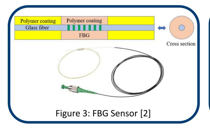
The Fiber Bragg Grating (FBG) sensor (Figure 3 and Figure 4) was chosen for this research due to its combination of high precision, long-term stability and resistance to corrosive environments.
