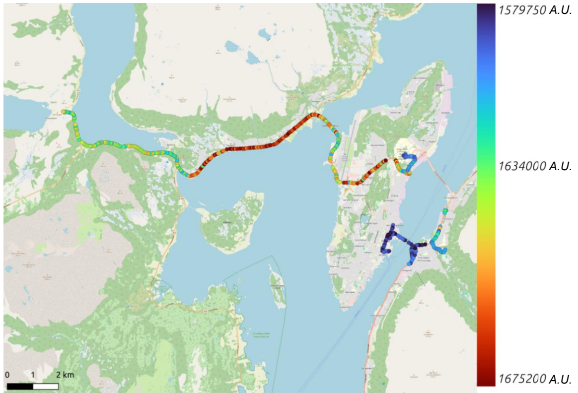
Fig. 22: The magnetic field values measured by the NV-based magnetometer before filtering over the course of a day during the polar circle excursion. An arbitrary unit was used, as the purpose of this figure is to show similarities in trends, and the bias magnet makes absolute measurements misleading.
