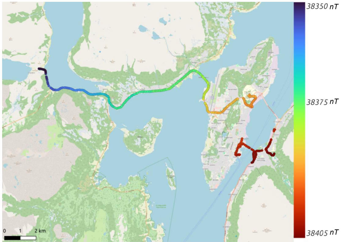
Fig. 24: The magnetic field values measured predicted by the CHAOS model for the same points as those displayed in Fig. 22 and Fig. 23 in nanotesla.
