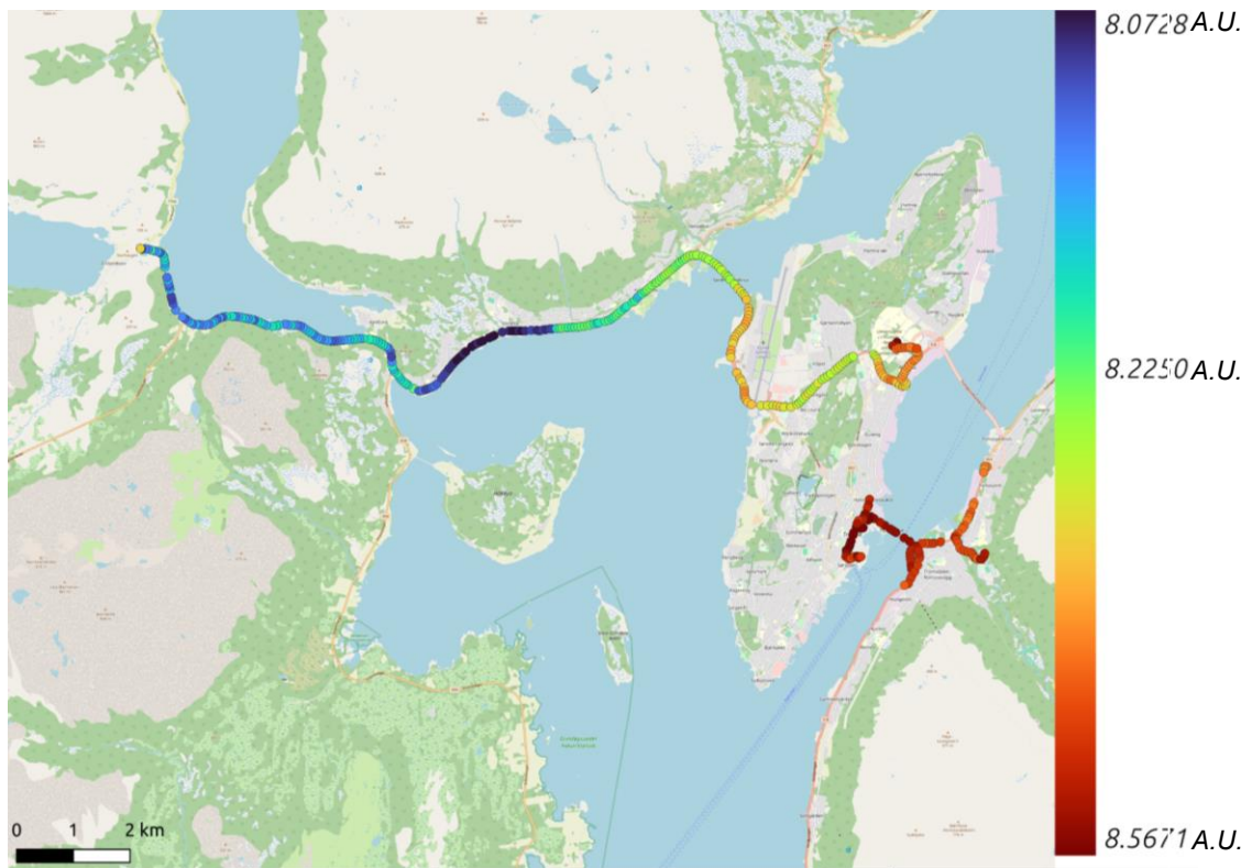
Fig. 23: The magnetic field values measured by the reference magnetometer before filtering over the course of a day during the polar circle excursion. An arbitrary unit was used, as the purpose of this figure is to show similarities in trends, and the bias magnet makes absolute measurements misleading.
