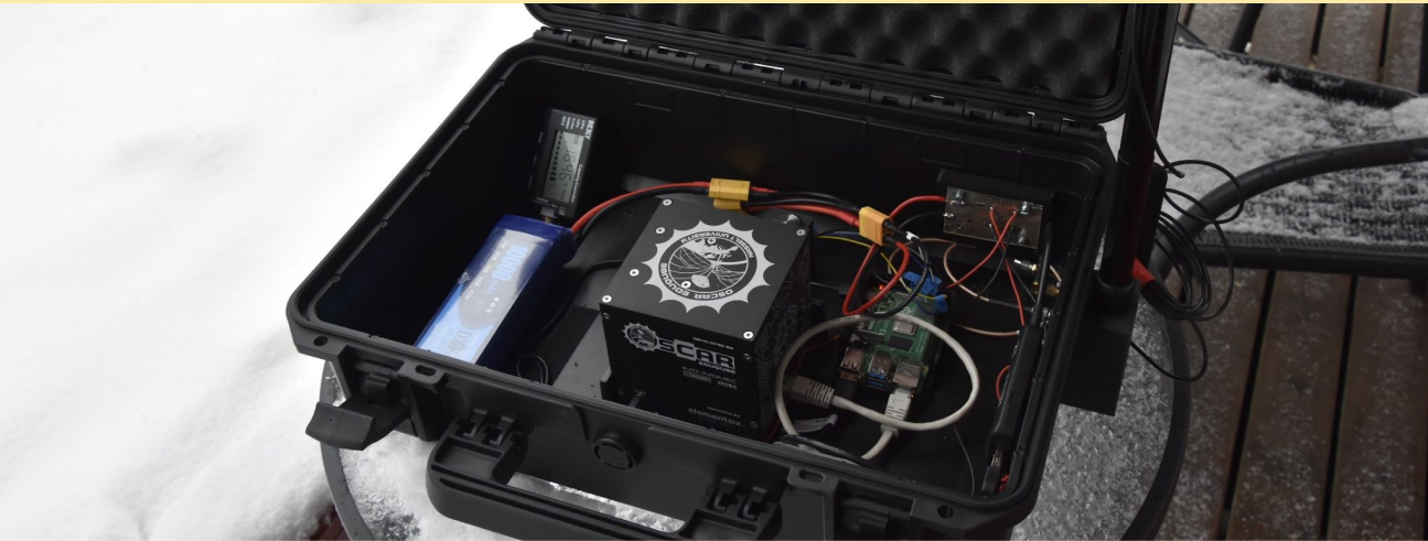
Figure 3: The mobile detector using an NV-magnetometer
