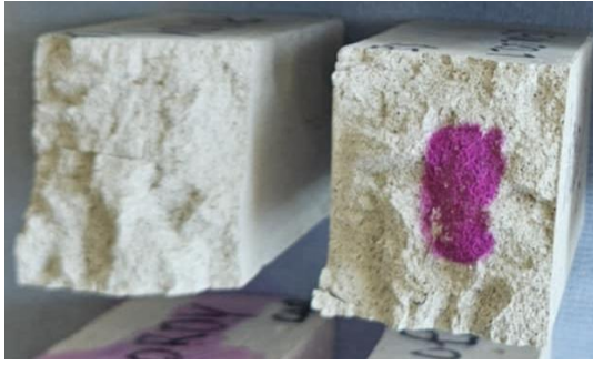
Figure 21: Carbonation depth CEM_00_CAR; CEM_00_REF
