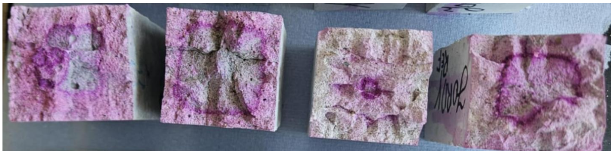
Figure 20: Carbonation depth CEM_15_CAR; CEM_15_REF; CEM_10_CAR; CEM_10_REF
