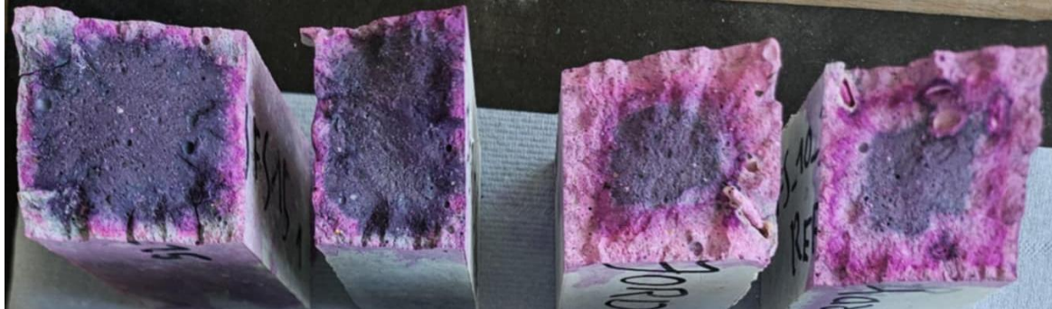
Figure 22: Carbonation depth BFS_15_CAR; BFS_15_REF; BFS_10_CAR; BFS_10_REF
