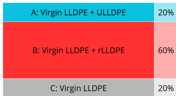
Figure 3.1: Layer structure of lab films
