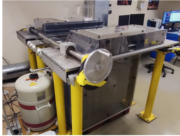
(a) Detector 10 with lead castle for small samples. (b) Detector 5 with lead castle for large samples.
