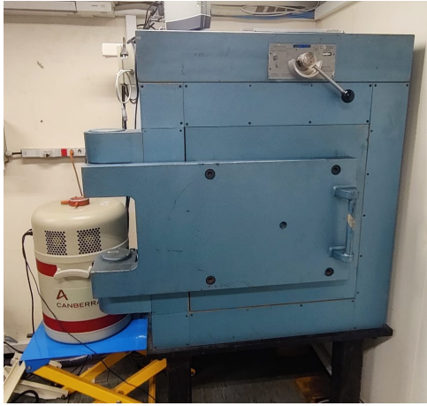
(a) Detector 10 with lead castle for small samples. (b) Detector 5 with lead castle for large samples.
