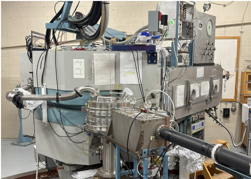
Figure 4.6: The Enge spectrometer at the HIAF facility. It is positioned on rails to rotate the spectrometer.
