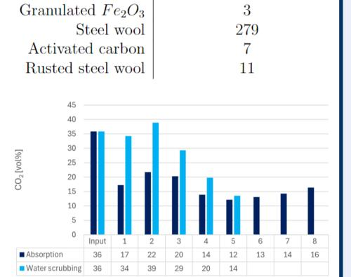
Figure 5: CO<sub>2</sub> concentration during the purification process
