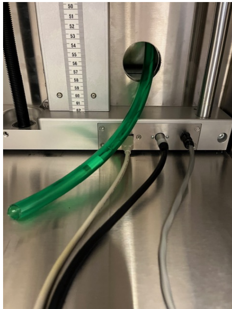
Figure 4.14: Testing the bending of the OFS in the MultiRad 225.
