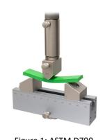
Figure 1: ASTM D790 standardized flexural test [1]
