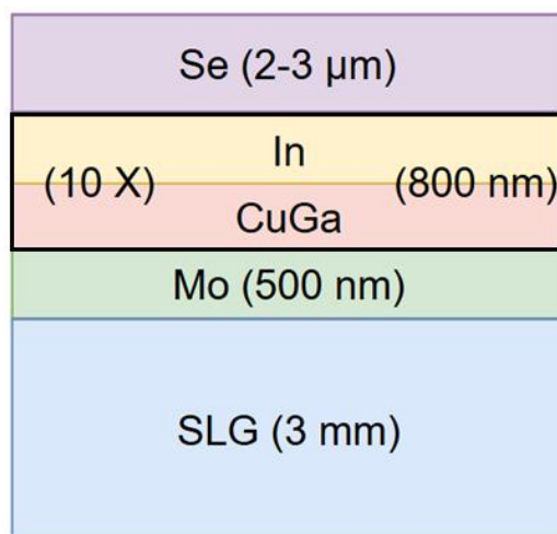
Figure 7: Metal layer stack after the sputtering step
