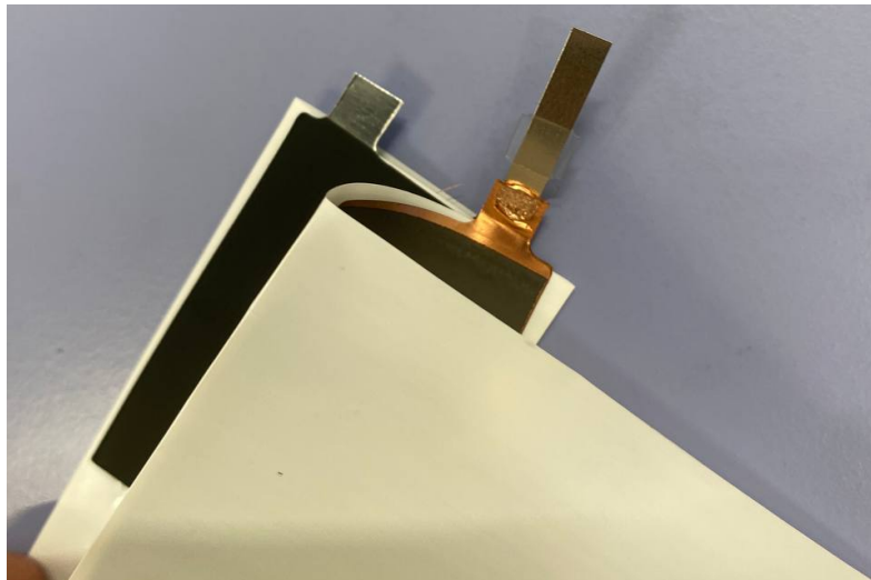
Figure 5.6: Close-up of the electrode stack showing the folded separator wrapping around the cathode and positioned between two anode layers.
