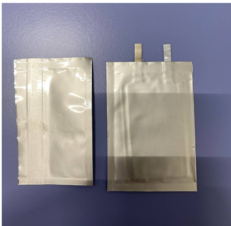
Figure 5.16: Excess pouch foil trimmed after final sealing.
