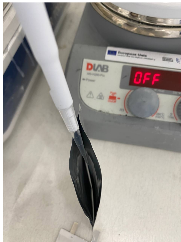
Figure 5.12: Dropping of electrolyte onto the electrode stack using a volumetric pipette.
