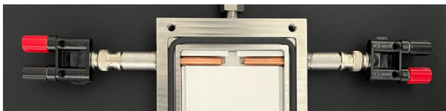
Figure 3.11: Internal view of the copper feedthrough connection system.
