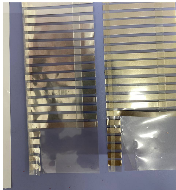
Figure 5.2: Current collector tabs for anode and cathode connection.
