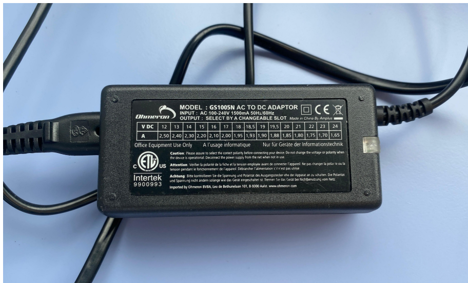
Figure 4.4: 24 V DC power supply with a maximum output current of 2 A.
