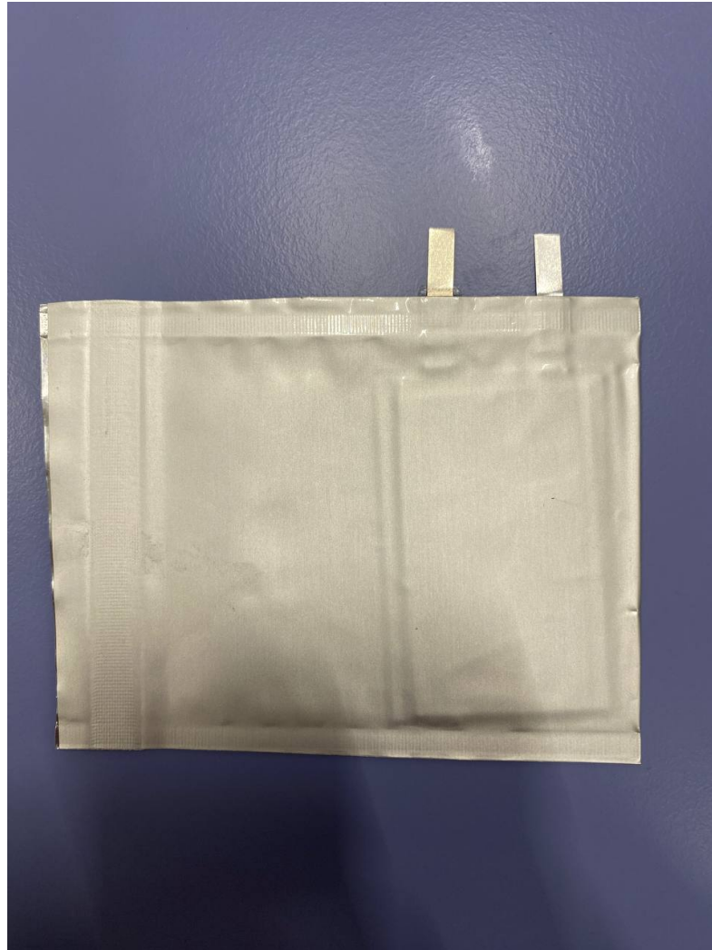
Figure 5.14: Fully sealed pouch cell after vacuuming.
