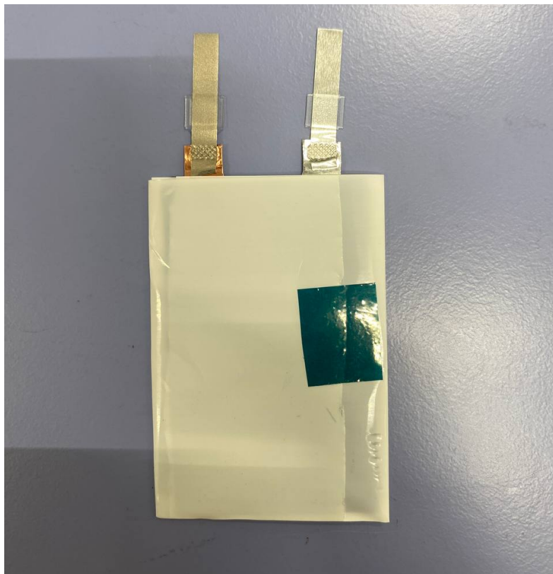
Figure 5.7: Completed electrode stack with polyimide tape holding the layers in position.
