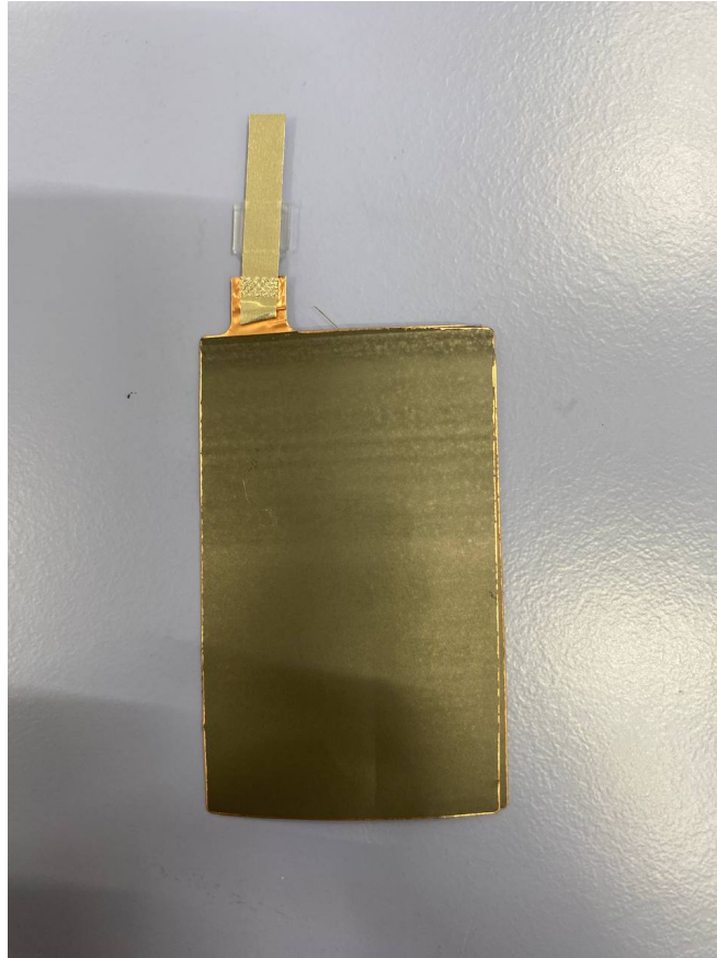
Figure 5.5: Placement of nickel tab on the anode electrodes.
