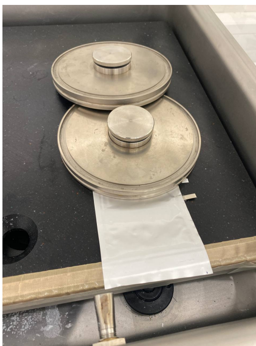
Figure 5.13: Pouch cell placed into a vacuum heat-sealer to evacuate air and close the final edge.
