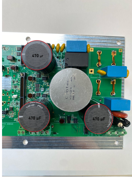
Figure 3.33: DC-link capacitance of 1410 \mu\text{F}
