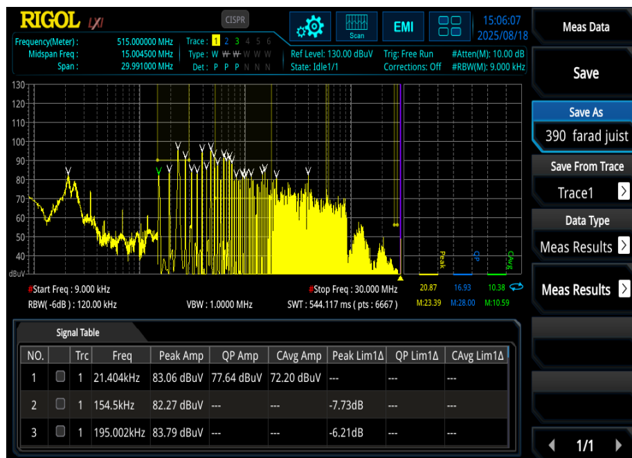
Figure B.4: EMI measurement of 390 \mu F capacitance
