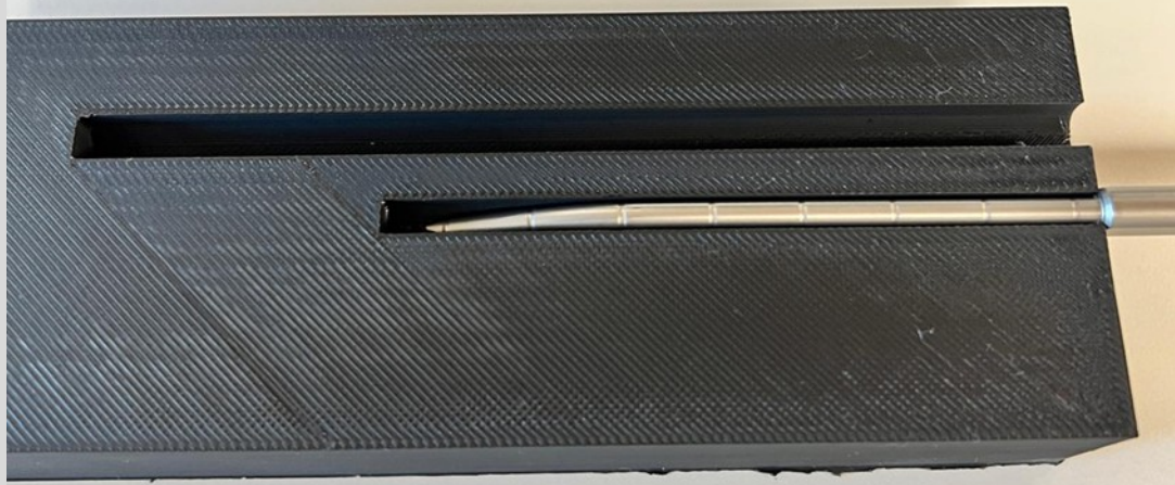
Figure 1: 3D-printed PLA phantom with applicator inside
