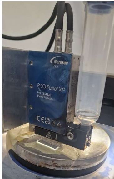
Figure 12: Experimental setup of the drop-on-demand jetting system
