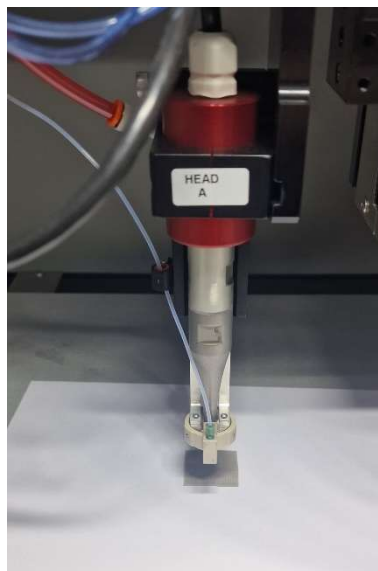
Figure 15: Ultrasonic spray coater head used for ultrasonic spray coating samples
