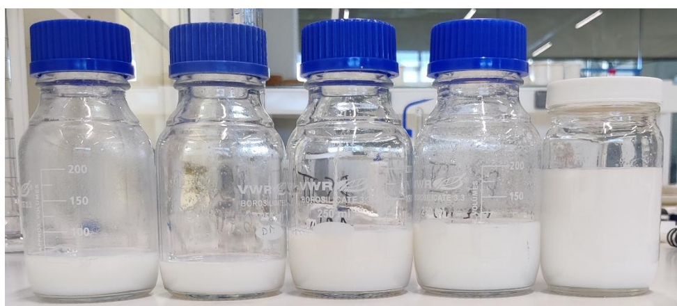
Figure S2. Picture of the obtained samples from the emulsion polymerizations of destabilized styrene. From left to right: PS1-2-3-4-5.
