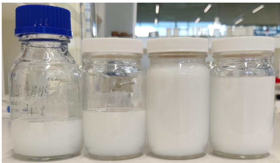
Figure S3. Picture of the obtained samples from the emulsion polymerizations of destabilized methyl methacrylate. From left to right: PMMA1-2-3-4.
