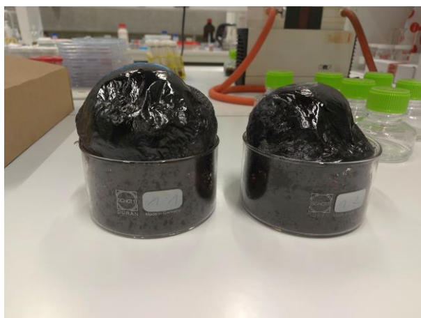
Figure S2: Inflated pre-calcined multi-metal product.
